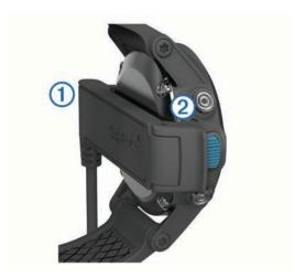
**4** Align the hinged side of the charger ② with the contacts on the back of the device.
