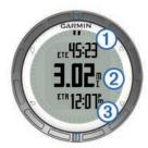
The device displays time to destination ①, distance to destination ②, and estimated time of arrival ③.
