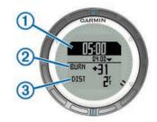
The race timer screen displays the race timer ①, time to burn ②, and distance to the start line ③.
