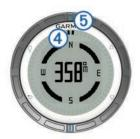
The two pointer marks ④ serve as a bearing pointer. The top orange mark ⑤ points in the direction you are facing.
