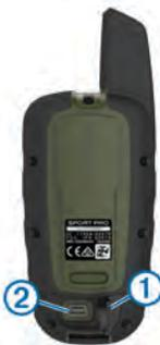
You should fully charge the battery before you use the device for the first time or whenever the battery is low. It is normal for the battery to discharge in approximately 7 to 10 weeks when the device is not in use. Charging a fully depleted battery takes about 2 hours.
