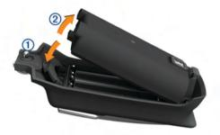
3 Insert four AA batteries, observing polarity.
