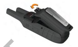
4 Turn the D-ring clockwise to secure the battery pack onto the device.
