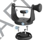
5 Place the swivel mount bracket ④ over the swivel base and secure it with the short knob ⑤.
