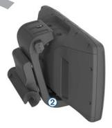
3 Tilt the device back until it snaps into place.
