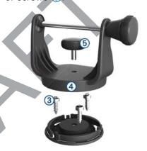
Place the swivel mount bracket 4 over the swivel base and secure it with the short knob 6.
