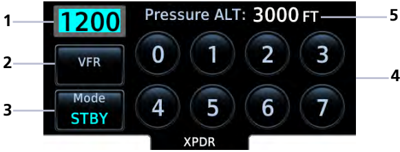
XPDR Control Panel
