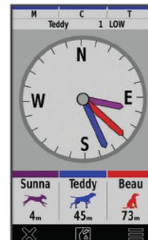
You can use the dog tracking compass to view the direction and distance to your dog, your vehicle, and any paired devices. The dog tracking compass also shows the dog's status, such as running or on point (*Dog Status Icons*, page 5). The color of the pointer corresponds to the color of the track.
