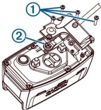
3 Remove the screw ② securing the VHF antenna to the back plate.
