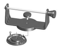
Secure the base and attach the mount
