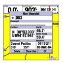
Highlight the position field and use the **ARROW KEYPAD** to enter the desired position coordinates.
