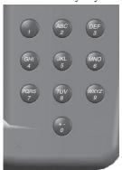
waypoint name. Use data entry keys in conjunction with the **ROCKER**. Press the key once to select the first letter on the key, twice to select the second letter on the key, three times to select the third letter on the key, or four times to select the number on the key. For keys 7, 8, and 9, press the key five times to select the number on the key. When you have selected the correct letter or number, pause, and the unit advances the cursor to the next character automatically.
