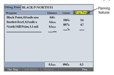
Press left or right on the ROCKER to select one of nine available planning features, including ETA (Estimated Time of Arrival at point), Fuel (to point), Leg Dist, Leg Fuel, Leg Time, Sunrise, Sunset (at point location), and Time To (point).
