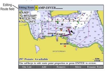
3. Use the **ROCKER** or data entry keys to change the route name, and press **ENTER** when finished.
