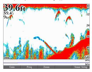
The sonar function window contains a right-to-left moving sonar image of the water beneath your boat. Items appear as they pass under the transducer. The most recent data is shown on the right side of the screen. The right side of the screen contains a scale reflecting the depth of the area being shown. The top-left corner shows the depth, water temperature, and speed through water (if equipped with a temperature or speed sensor).
