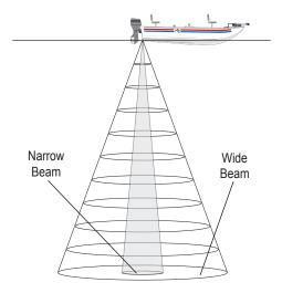
The wide beam is more helpful in shallow water, because it gives you a much wider view of objects in the water, including areas beyond the sides of your boat. At a 30-foot depth, the wide beam covers the area of approximately a 20-foot circle.
