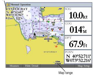
Use the **Up** and **Down** keys and the **ROCKER** to select zoom ranges and move the map pointer. Two basic map operating modes, Position mode and Pointer mode, determine what cartography (map data) is shown on the Map Page. Position mode pans the cartography to keep the current position marker within the display area, whereas Pointer mode pans the cartography to keep the map pointer within the display area.
