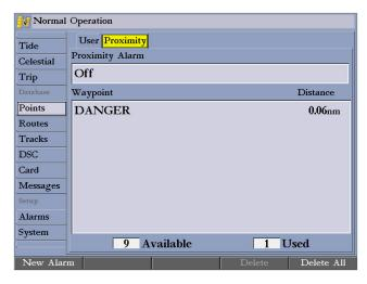
The total number of stored and available proximity waypoints appears at the bottom of the Proximity sub tab, with the stored waypoints arranged in alphanumeric order.
