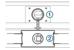
3 Secure the antenna to the pedestal using the included hex bolts (3) and spring washers (4).
