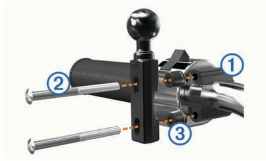
**NOTE:** Both 1/4 in. standard and M6 bolts are included. Match the size of the factory bolts on your clutch/brake-clamp bracket.
