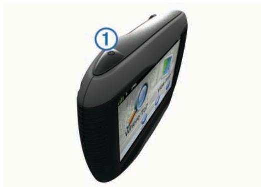
**NOTE:** If you hold the Power key for less than 5 seconds, the device enters sleep mode ([page 3](#)).
