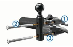
**NOTE:** Both 1/4 in. standard and M6 bolts are included. Match the size of the factory bolts on your clutch-clamp or brake-clamp bracket.
