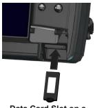
Data Card Slot on a GPSMAP 492/498
