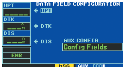
Figure 8-78 Upper Data Field Highlighted
