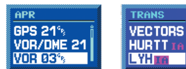
Figure 5-12 Approach and Transitions Windows
