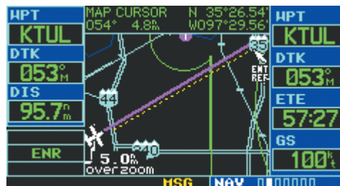
Figure 2-21 Using Pointer to Measure Distance and Bearing
