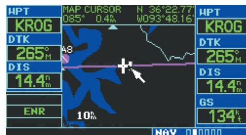
Figure 6-39 Activate Panning Function
