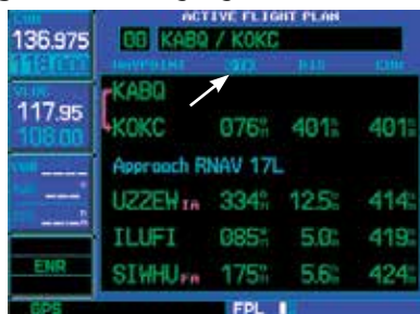
Changing fields for the active flight plan.
