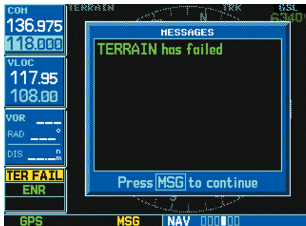
“TERRAIN has failed” message
