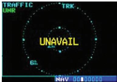
Traffic With GDL 88 and Invalid Heading or Track
