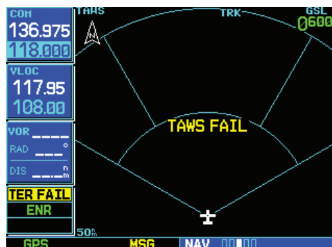
TAWS FAILED Display
