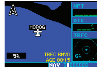
Thumbnail Traffic displayed on the GNS 430W.
