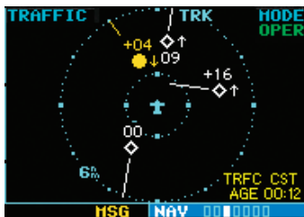
Traffic Age Indication showing “traffic coasting”.
