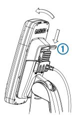
2 Tilt the device forward, and lift it out of the cradle.
