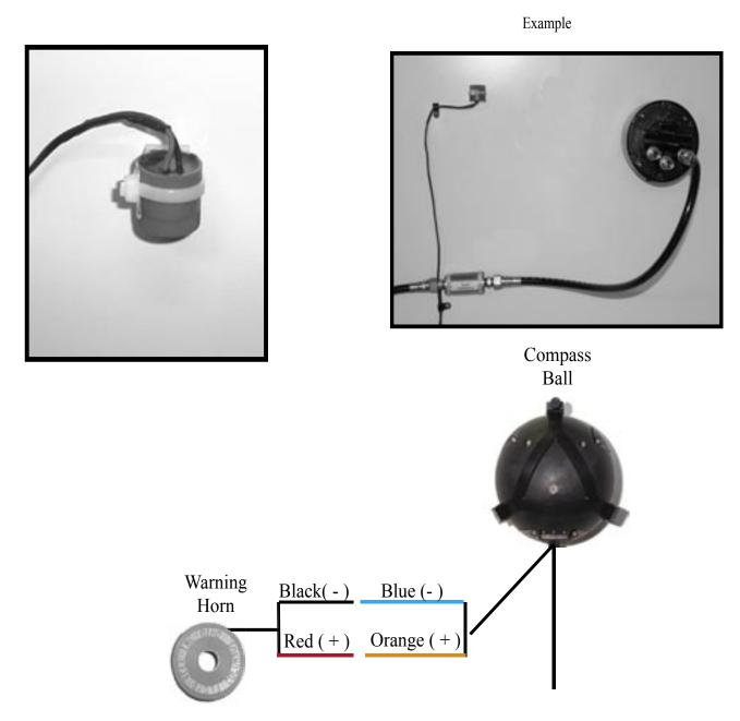
The electrical connections for the warning horn are made at the compass ball. The Black ( - ) and Red (+ ) wire on the warning horn connect to the Blue (- ) and Orange (+) coming from the Compass Ball. Mount the warning horn using the cable tie and mount with screw included in your installation kit. The wire for the warning horn can be extended using shielded two conductor wire.
