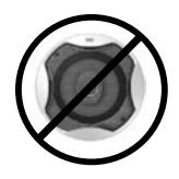
Do not mount the compass near magnetic devices such as radio speakers or electric motors such as the autopilot pump motor.
