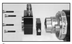
4) Insert the new longer screws that came with the kit, lining up the holes in the unbalanced valve and the pump motor.
