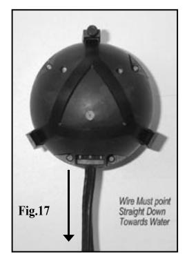
**Step Three: Adjusting Compass Ball**
