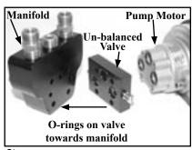
3) Place the unbalanced valve between the pump motor and the manifold with the O-rings facing the manifold. Six O-rings are required and are supplied in the kit. Three (3) are in the pump motor and three (3) are in the unbalanced valve.
