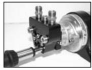
5) Tighten all four screws apply a thread locking compound and tighten to 35 in lbs.
