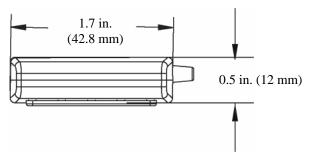
Figure 2. GPS 20x Side View
