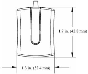
Figure 1. GPS 20x Top Case Dimensions
