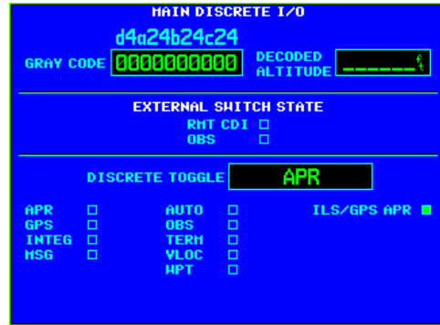
Figure 5-8. MAIN DISCRETE I/O Page
