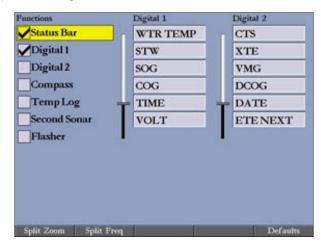
Using the ROCKER, highlight the function you want to add or remove, and press ENTER. Only functions with a check mark in the check box next to them appear on the Sonar Page.
