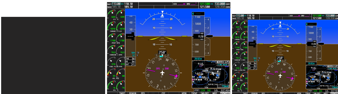
Figure 3-10. Manual Reversion with pilot PFD failure
