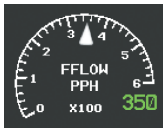
Figure 3-9 Fuel Flow Gauge
