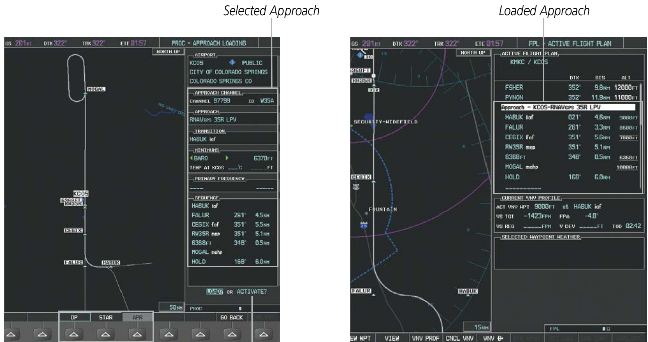
Procedure Loading Page Selection Softkeys LOAD or ACTIVATE? Annunciation Figure 5-100 Approach Loading
