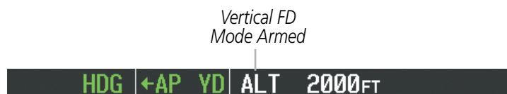
Figure 7-10 Vertical Flight Director Mode Armed
