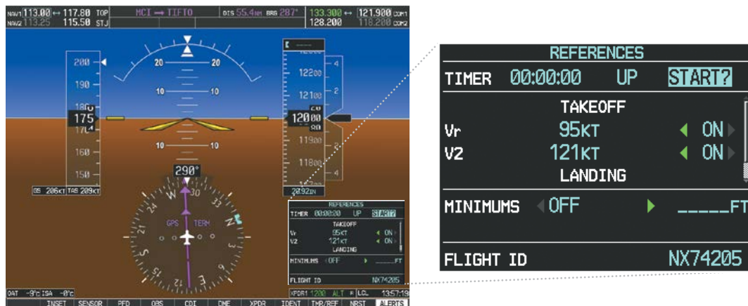
Figure 1-39 Generic Timer (PFD Timer/References Window)
