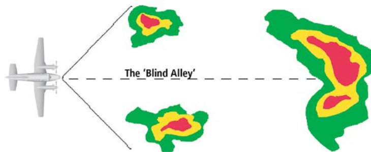
Figure 6-99 The Blind Alley - Horizontal Scan
