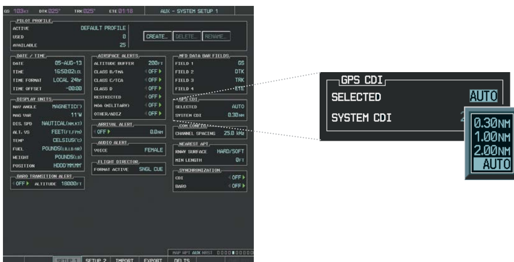
Figure 2-29 System Setup Page, GPS CDI Settings
