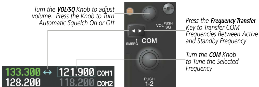
Figure 4-7 COM Frequency Tuning
