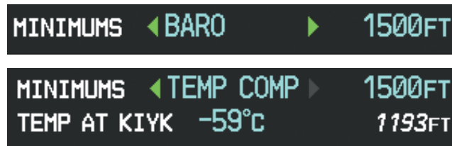
Figure 2-49 BARO and TEMP COMP MDA/DH
