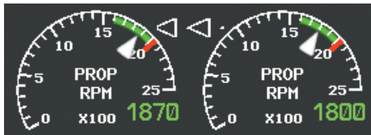
Figure 3-7 Propellers Out of Sync (greater than or equal to 50 rpm)
