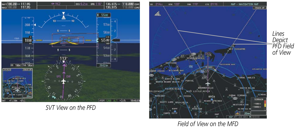
Figure 8-13 PFD and MFD Field of View Comparison
