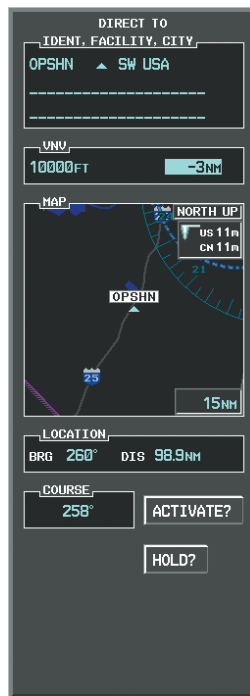
Figure 5-129 Enter VNV Offset Distance
