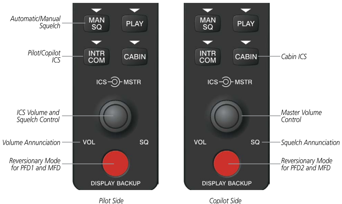
Figure 4-52 Audio Panel Controls
