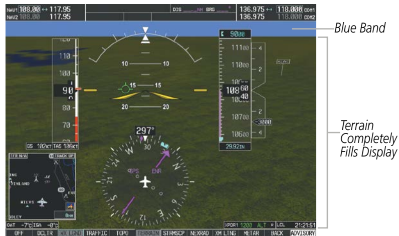
Figure 8-130 Blue Sky Bar with Full Display Terrain
