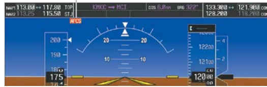
Figure A-8 AFCS System Status Field
