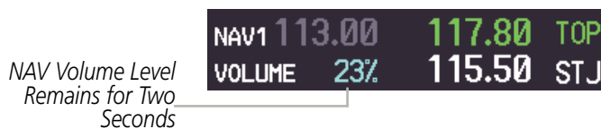
Figure 4-26 NAV Volume Level
