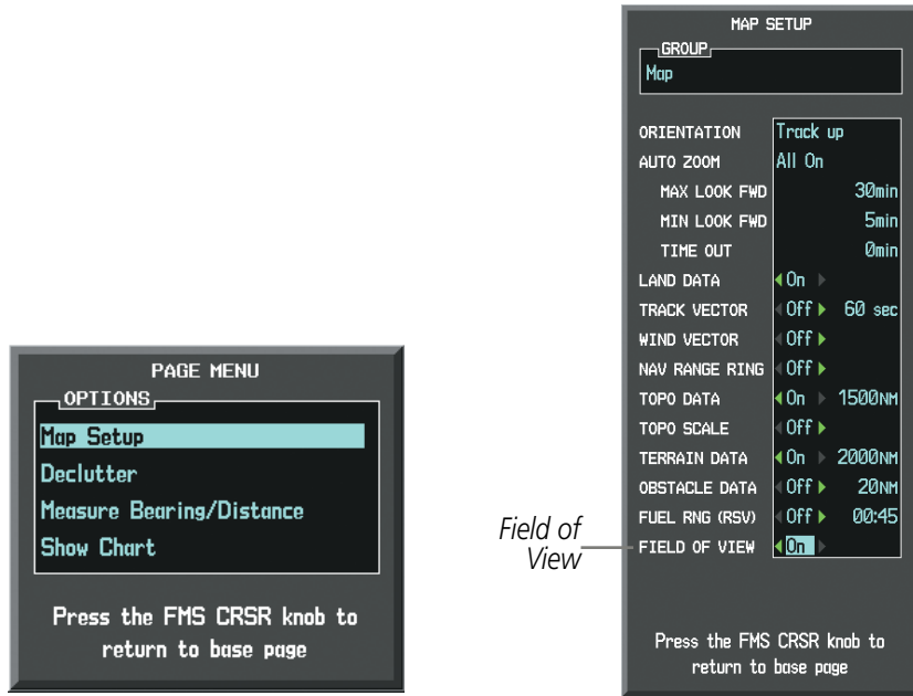
Navigation Map Page OPTIONS Menu Map Setup Menu, Map Group, Field of View Option
