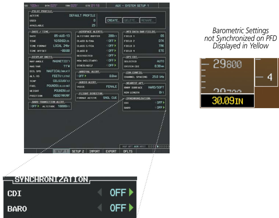
Figure 2-13 System Setup Page, Barometric Pressure Synchronization
