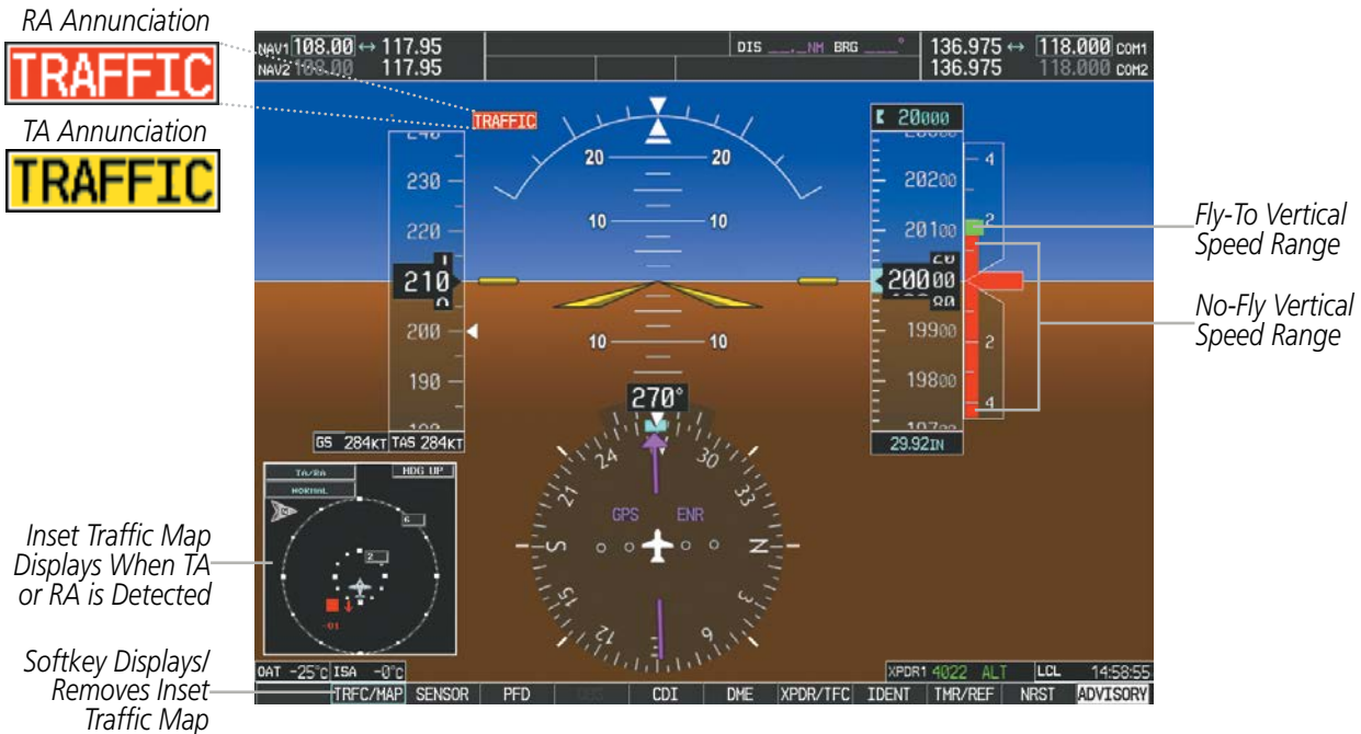
Figure 6-189 Traffic Annunciation with Resolution Advisory (PFD)
