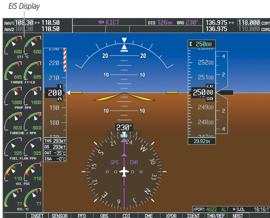
Figure 3-12 Reversionary Mode (200/B200)
