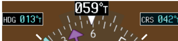
Figure 2-21 Heading and Course Indications (True)
