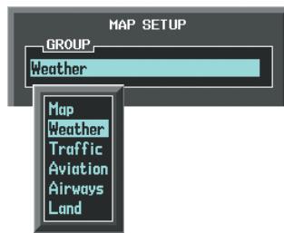
Figure 6-59 Navigation Map Page Setup Menu
