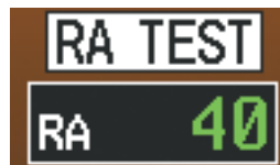
Figure 2-55 Radar Altimeter with Test Annunciation
