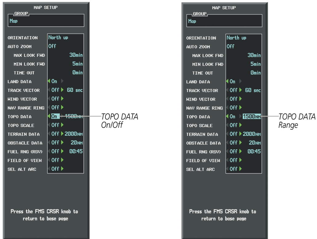
Figure 5-15 Navigation Map Setup Menu - TOPO DATA Setup
