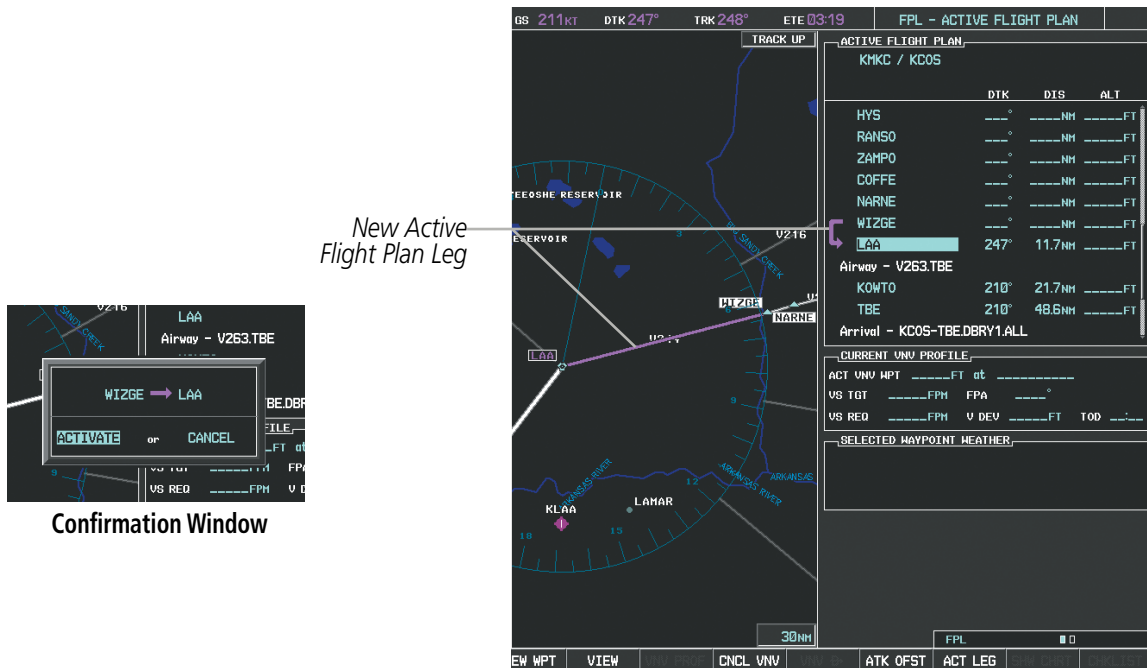
Figure 5-85 Active Flight Plan Page - New Active Leg
