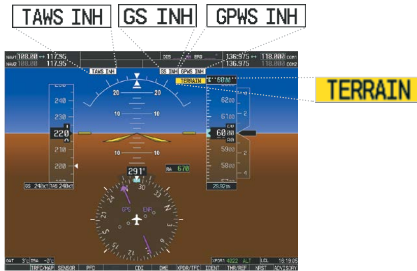
PFD with TAWS-A Annunciations
