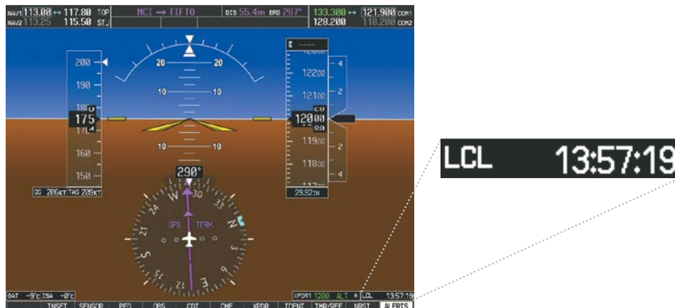
Figure 1-33 System Time (Local 24-hr Format)
