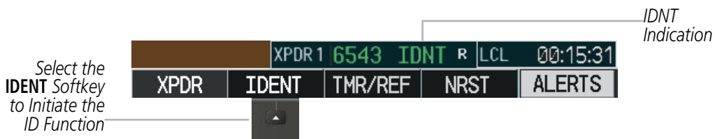
Figure 4-47 IDENT Softkey and Indication
