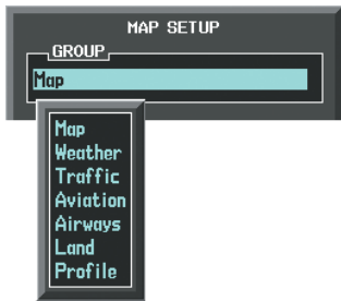
Figure 6-82 Navigation Map Page Setup Menu
