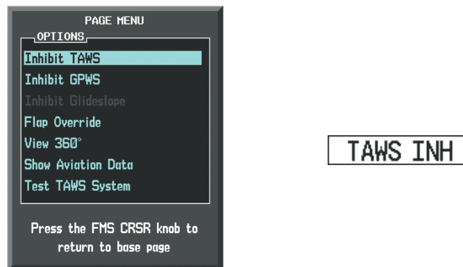
Figure 6-145 TAWS-A Page Menu and Inhibit Annunciation
