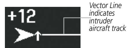
Figure 6-167 Intruder Traffic with ADS-B Directional Information and Track
