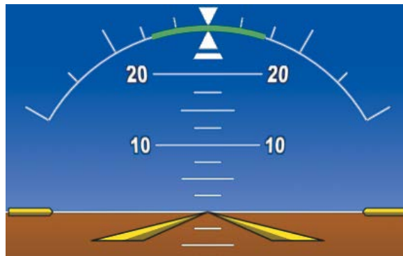
Figure 7-29 Low Bank Mode Limits
