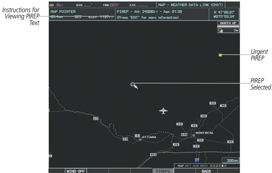
Figure 6-84 PIREPs on the Weather Data Link (CNXT) Page
