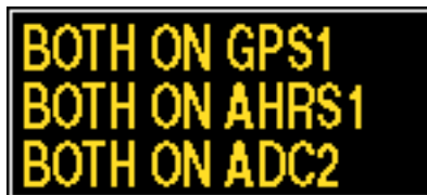
Figure 2-41 Reversionary Sensor Window
