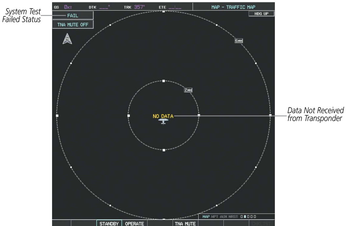
Figure 6-165 TIS Power-up Test Failure
