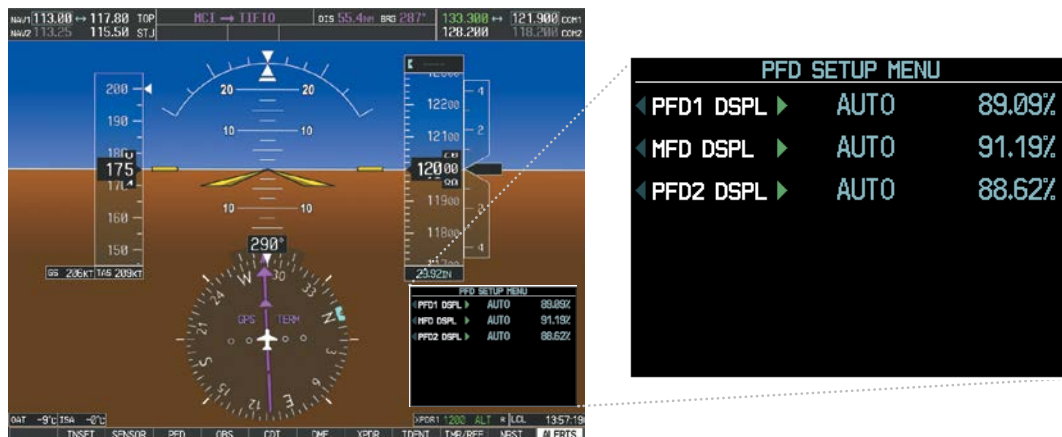
Figure 1-43 PFD Setup Menu
