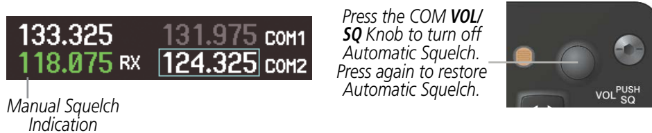
Figure 4-18 Overriding Automatic Squelch
