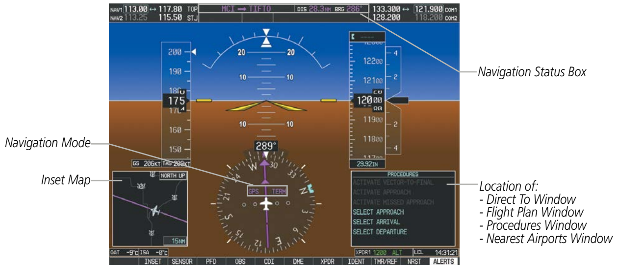
Figure 5-1 GPS Navigation Information on the PFD
