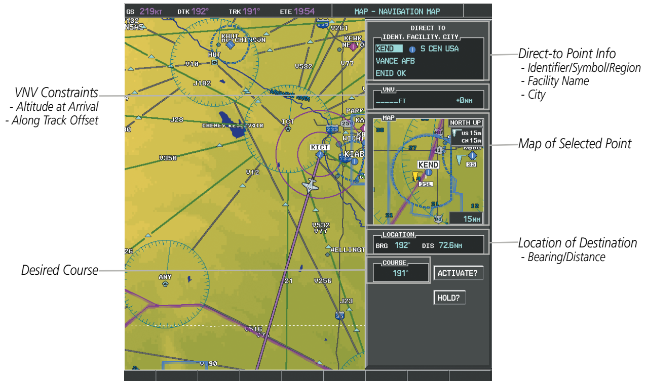
Figure 5-51 Direct-to Window - MFD
