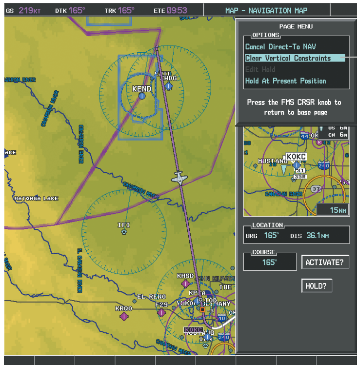
Figure 5-55 Direct-to Window - Clearing Vertical Constraints
