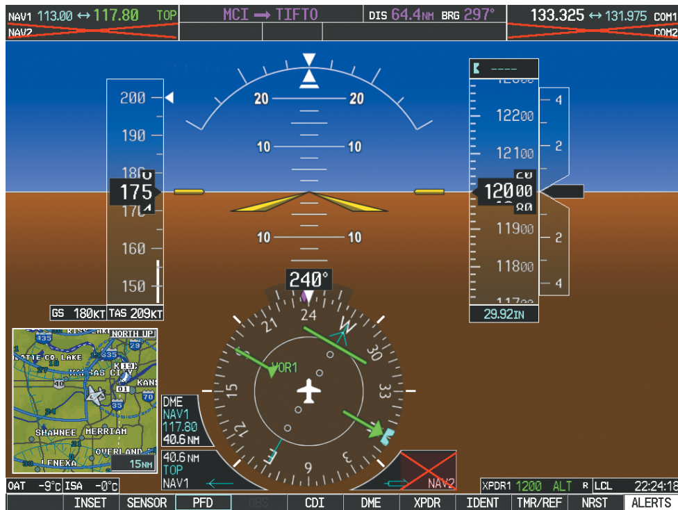
Figure 4-57 PFD1 Display after PFD2 Failure
