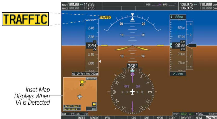
Figure 6-182 Traffic Annunciation (PFD)
