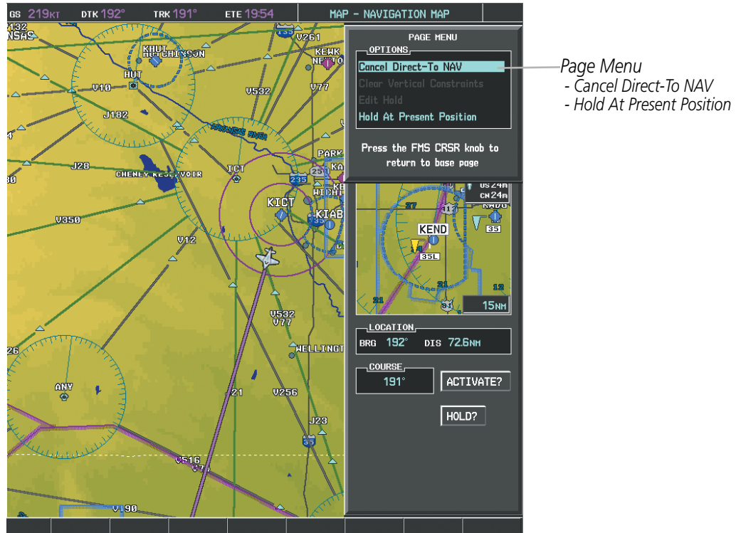
Figure 5-54 Direct-to Window - Cancelling Direct-to Navigation
