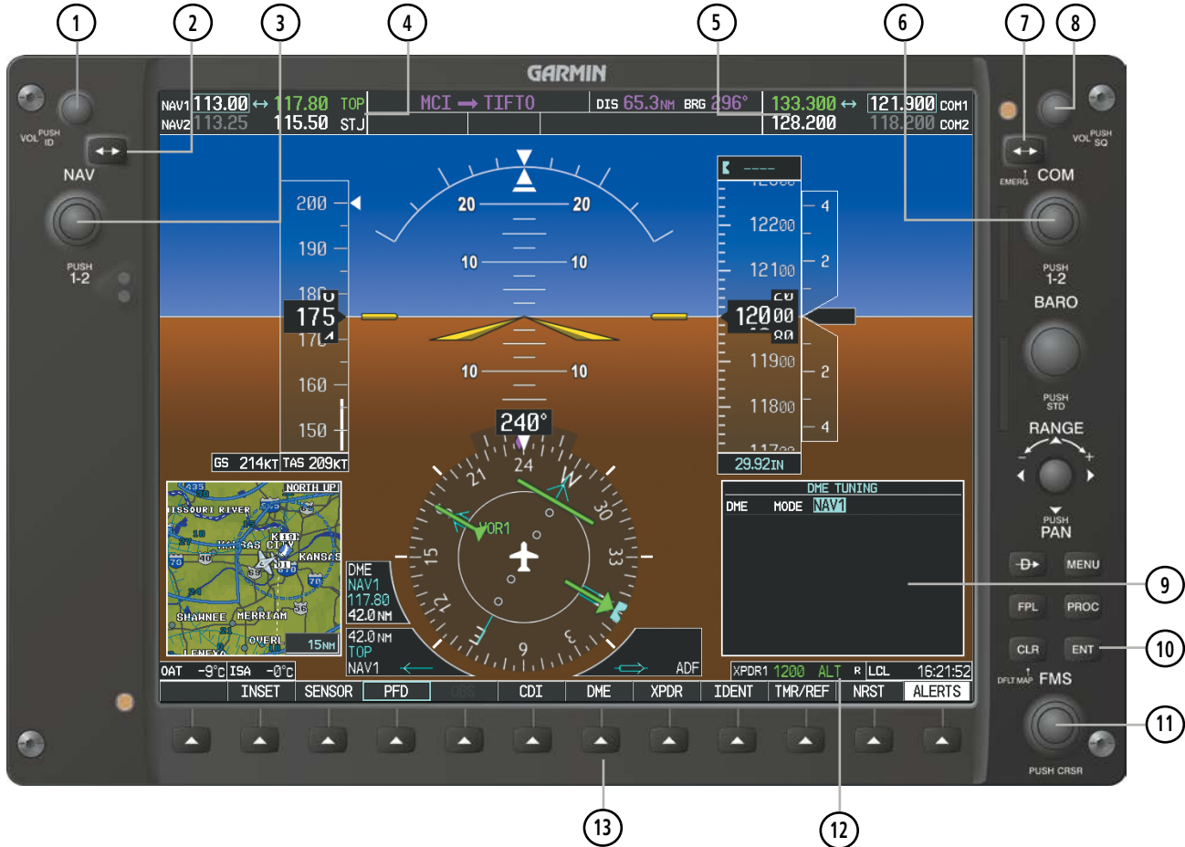
Figure 4-1 PFD Controls, NAV/COM Frequency Tuning Boxes, and DME Tuning Window
