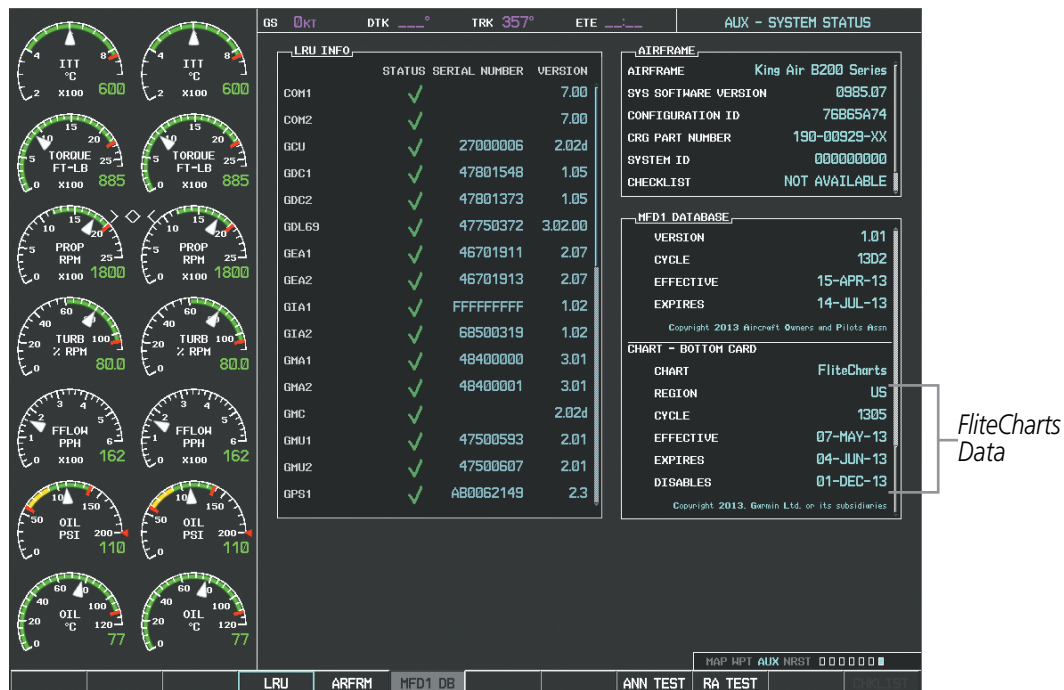
Figure 8-70 AUX – System Status Page, FliteCharts Current and Available
