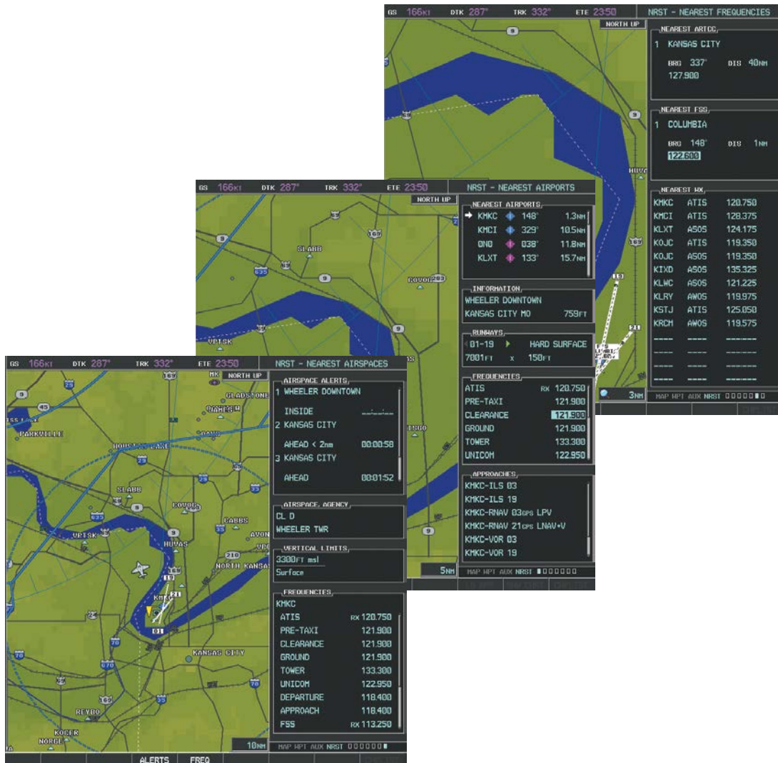
Figure 4-15 NRST – Nearest Airspaces, NRST – Nearest Airports, and NRST – Nearest Frequencies Pages
