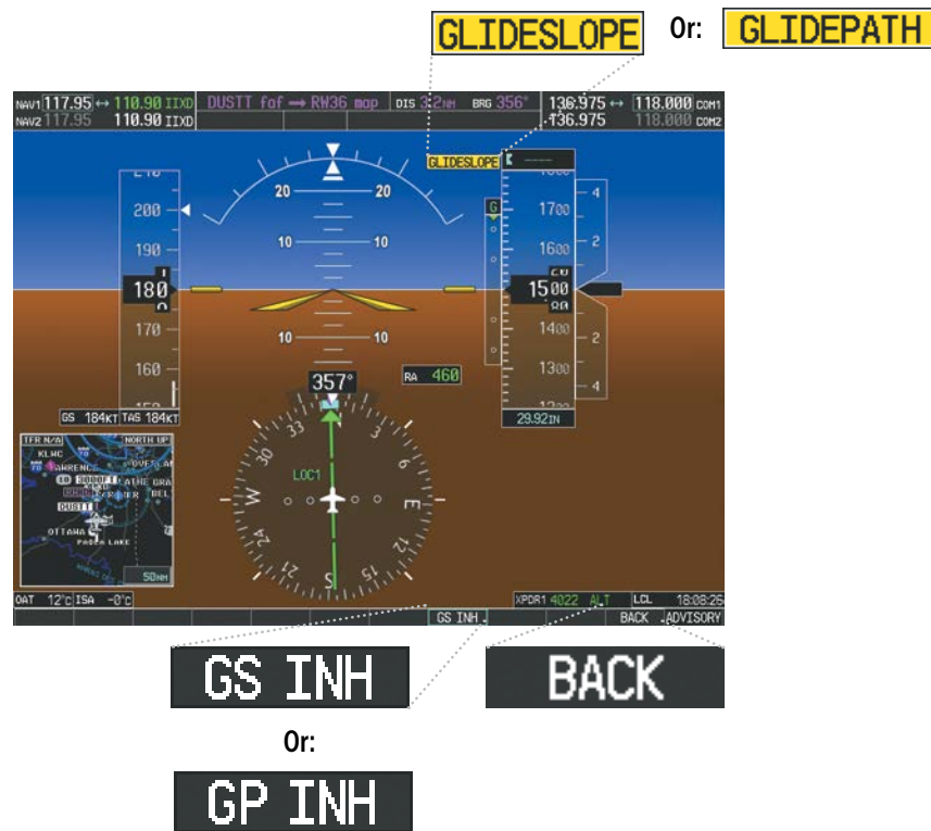
Figure 6-156 GSD Glideslope Alert and PFD Softkeys
