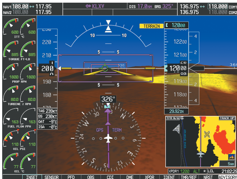
Figure 8-128 SVT Reversionary Mode
