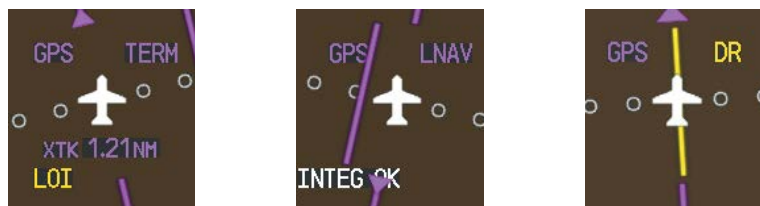
Figure 2-56 Example HSI Annunciations
