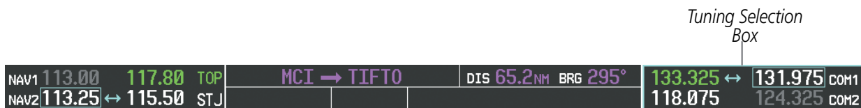
Figure 4-4 Frequency Tuning with the Control Unit
