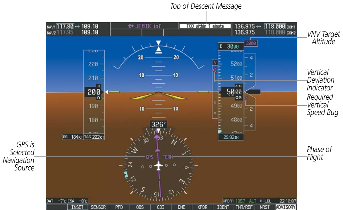
Figure 2-37 Vertical Navigation Indications (PFD)
