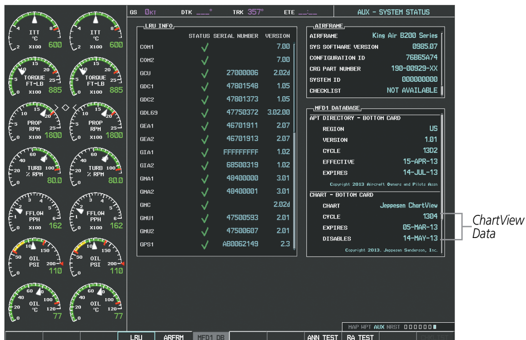
Figure 8-47 AUX – System Status Page, ChartView Current and Available
