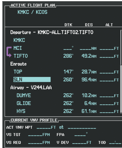
Figure 5-116 TOP Inserted into the Flight Plan
