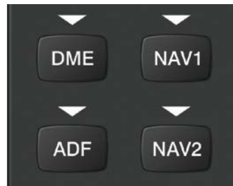
Figure 4-21 Selecting a NAV Radio Receiver
