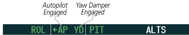
Figure 7-36 Autopilot and Yaw Damper Engaged
