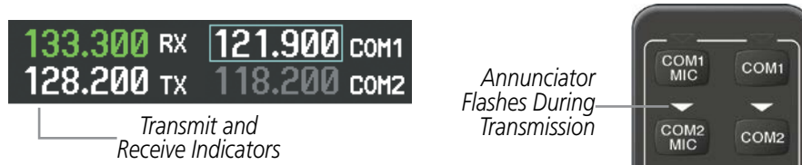
Figure 4-6 COM Radio Transmit and Receive Indications
