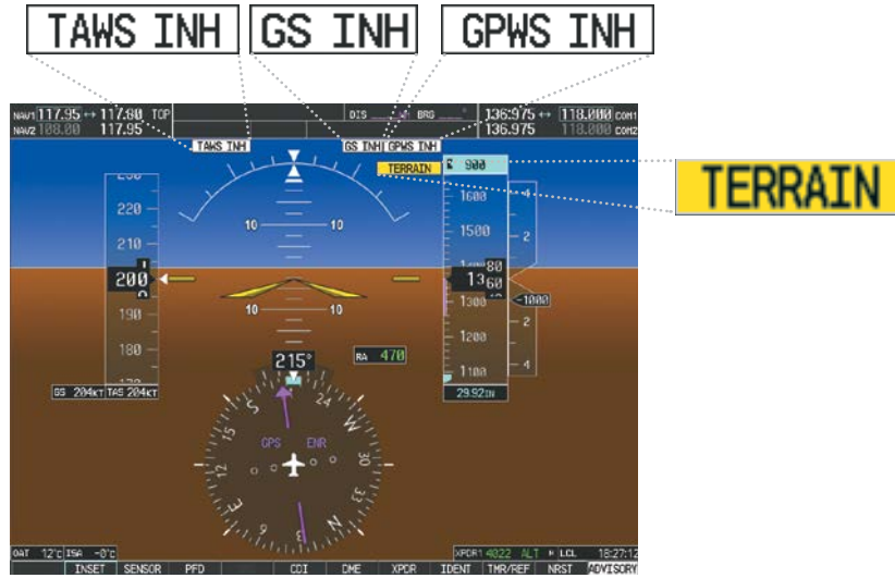
Figure 2-45 Example TAWS-A Annunciations
