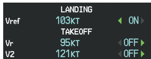
Figure 2-6 Takeoff and Landing Vspeeds (Timer/References Window)
