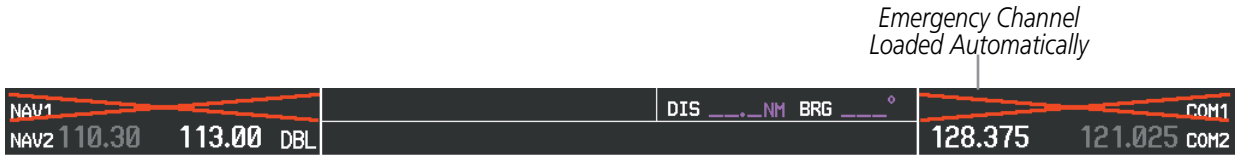
Figure 4-56 Frequency Section of PFD2 Display after PFD1 Failure
