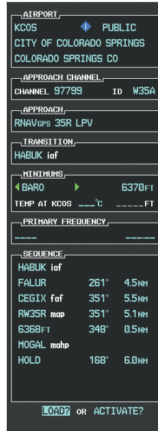
Figure 5-134 Barometric Minimums Set
