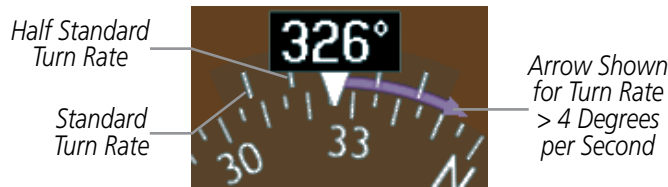
Figure 2-23 Turn Rate Indicator and Trend Vector
