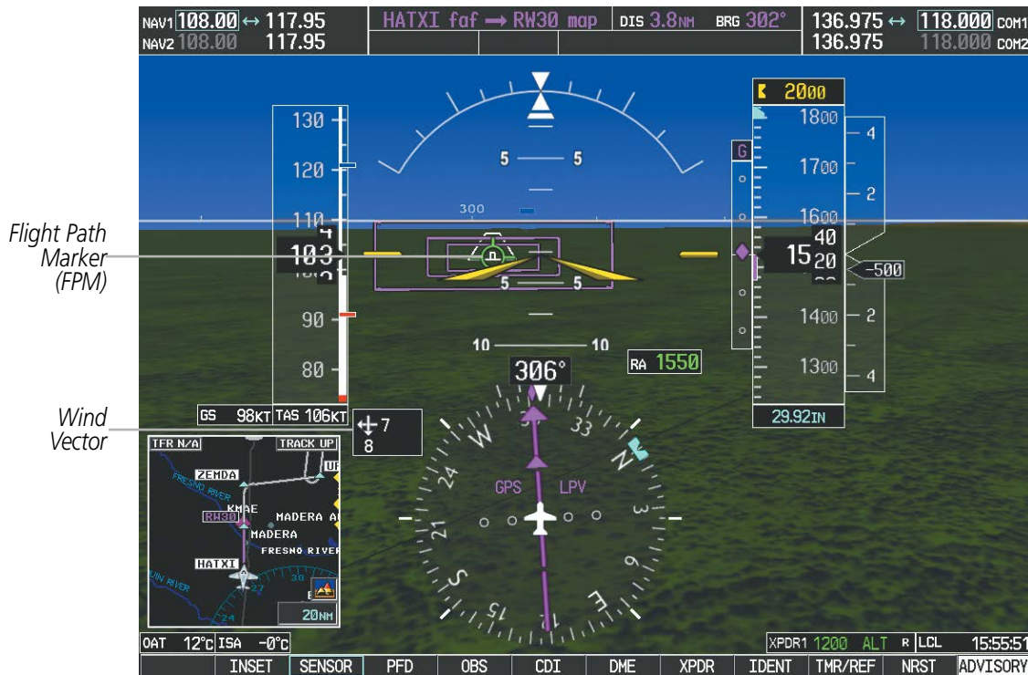
Figure 8-7 Flight Path Marker and Pathways
