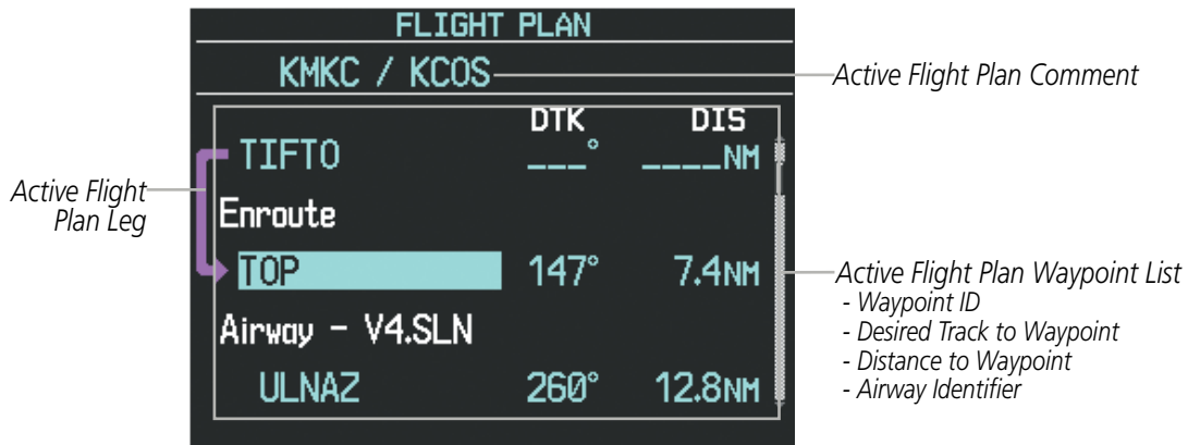
Figure 5-57 Active Flight Plan Window on PFD
