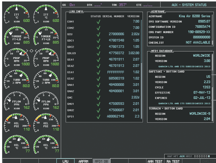
Figure 8-18 AUX – System Status Page, SafeTaxi Current Information
