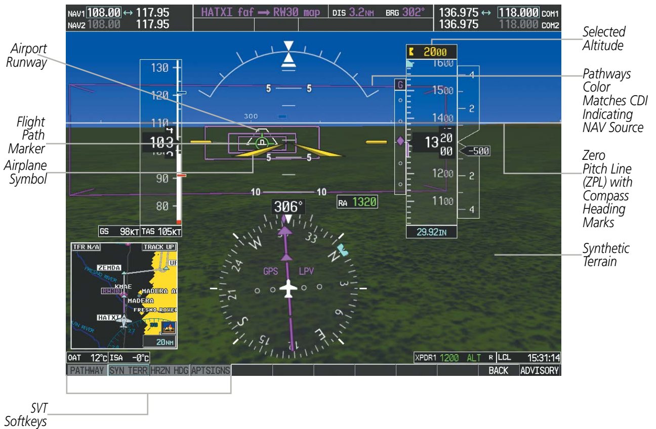
Figure 8-3 SVT on the Primary Flight Display
