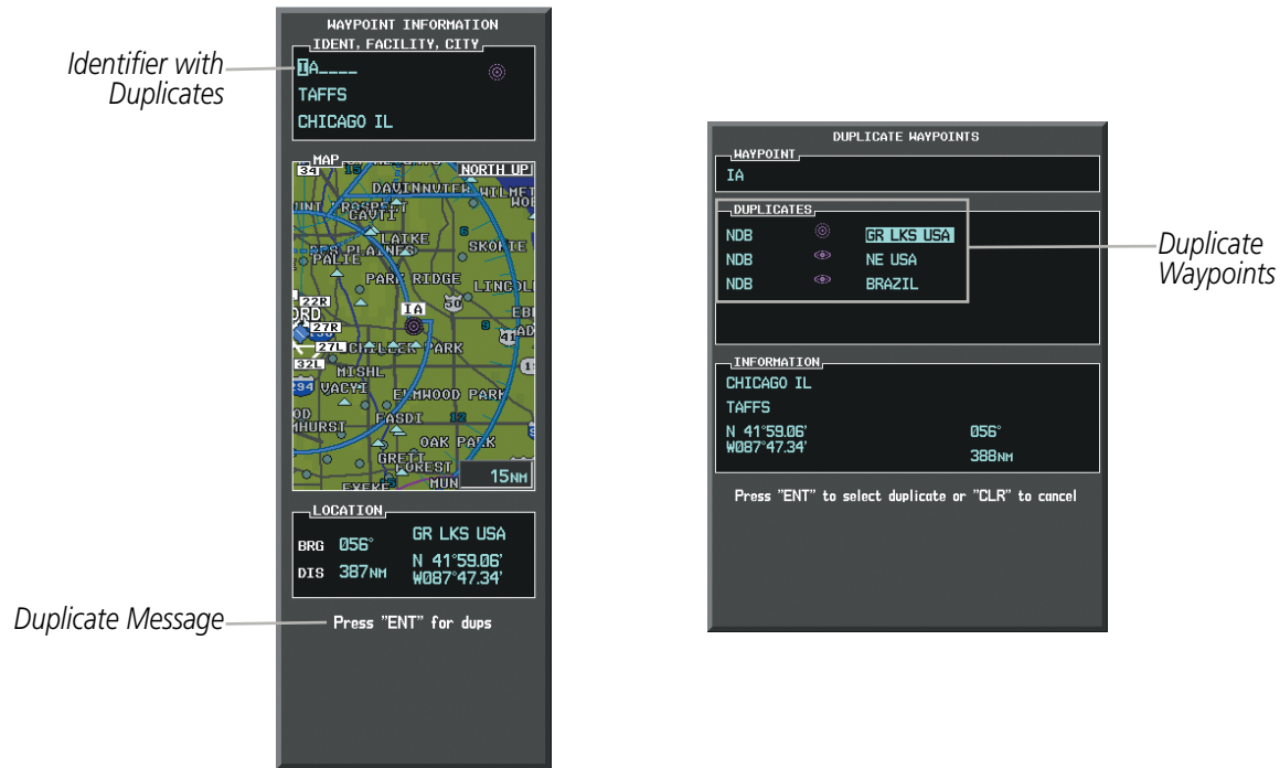
Figure 5-32 Waypoint Information Window - Duplicate Identifier
