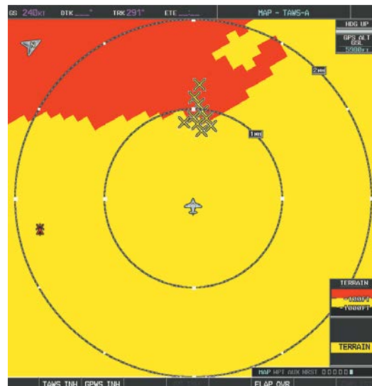
MFD TAWS-A Page with Alert Annunciation
