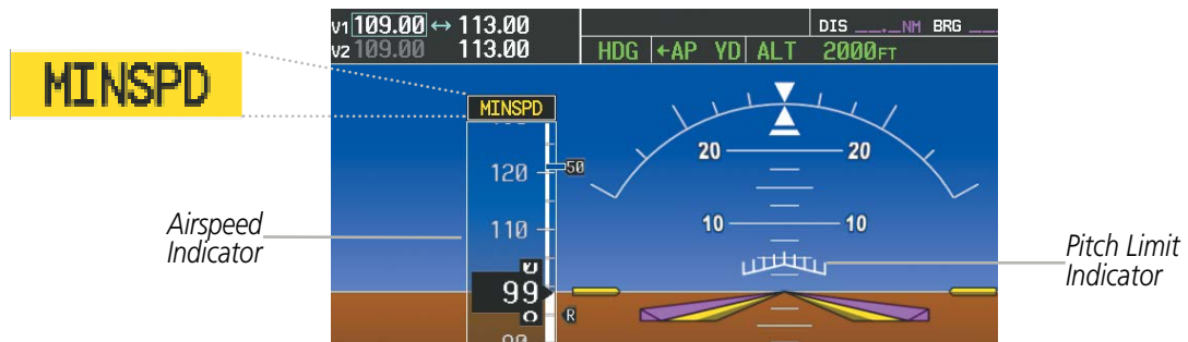
Figure 7-7 MINSPD Annunciation and Pitch Limit Indicator
