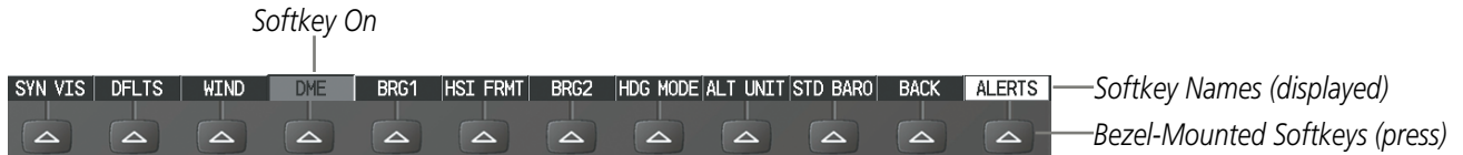
Figure 1-15 Softkeys (Second-Level PFD Configuration)
