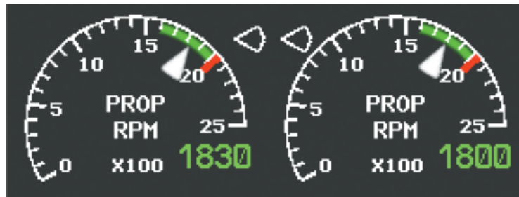
Figure 3-6 Propellers Out of Sync (less than 50 rpm)
