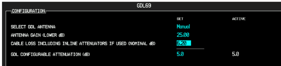
Figure 3-24, GDL 69 Cable Loss
