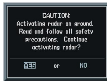
Figure 10-29 Confirming Activating Radar
