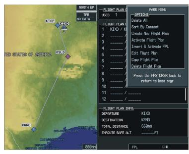
Figure 5-69 Invert and Activate a Flight Plan
