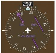
Figure 5-87 Assigned Heading of 290°
