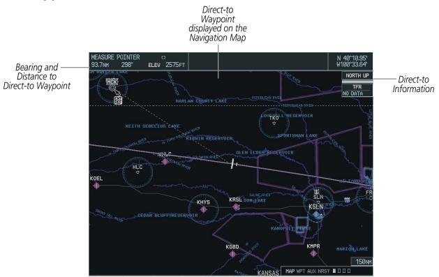
Figure 5-32 Direct-to Navigation Using Map Panning
