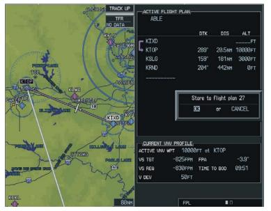
Figure 5-68 Storing a Flight Plan
