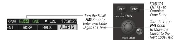
Figure 4-37 Entering a Code with the FMS Knob
