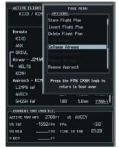
Figure 5-79 Collapse Airway Feature
