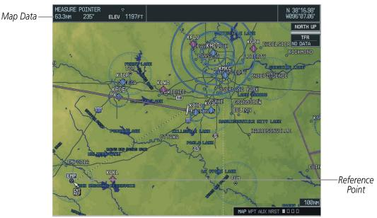
Figure 5-18 Measuring Bearing and Distance
