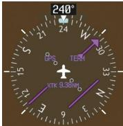
Figure 5-86 Assigned Heading of 240°
