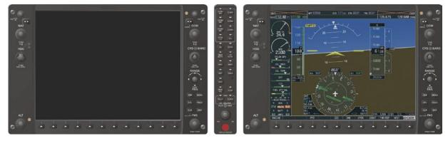
Figure 1-9 Reversionary Mode (Failed PFD)
