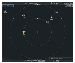
Figure 6-60 Self Test OK Display
