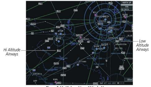
Figure 5-11 High and Low Altitude Airways
