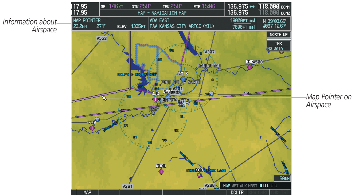
Figure 5-10 Navigation Map - Map Pointer on Airspace
