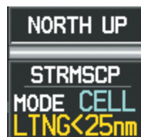
Figure 6-42 Lightning Display Range Annunciation
