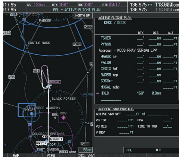
Figure 5-140 Establishing the Holding Pattern
