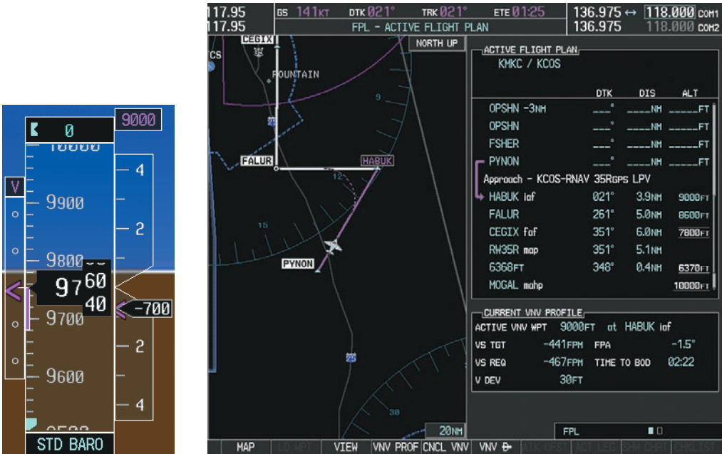
Figure 5-136 Descending Turn to the Initial Approach Fix (IAF)
