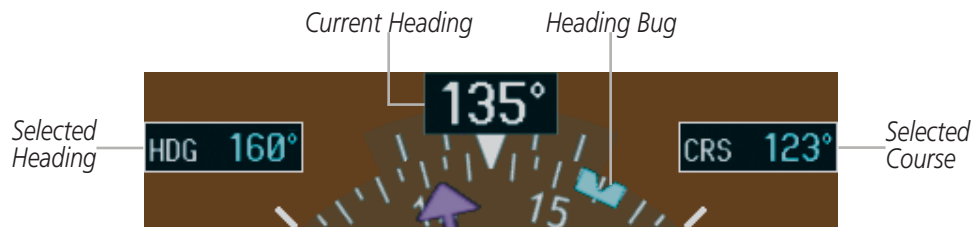
Figure 2-13 Heading and Course Indications (Magnetic)
