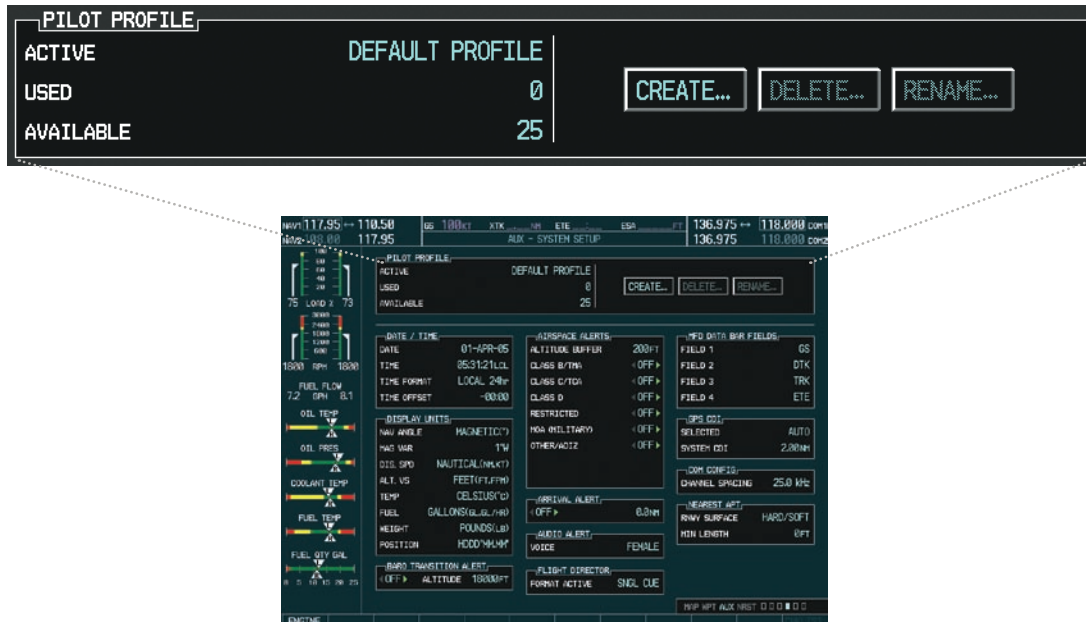
Figure 1-33 Pilot Profile Settings (AUX - System Setup Page)
