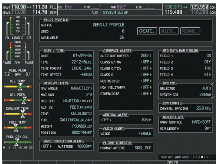
Figure 2-21 GPS CDI Settings (AUX-System Setup Page)
