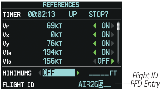
Figure 4-45 Timer/References Window, Entering Flight ID
