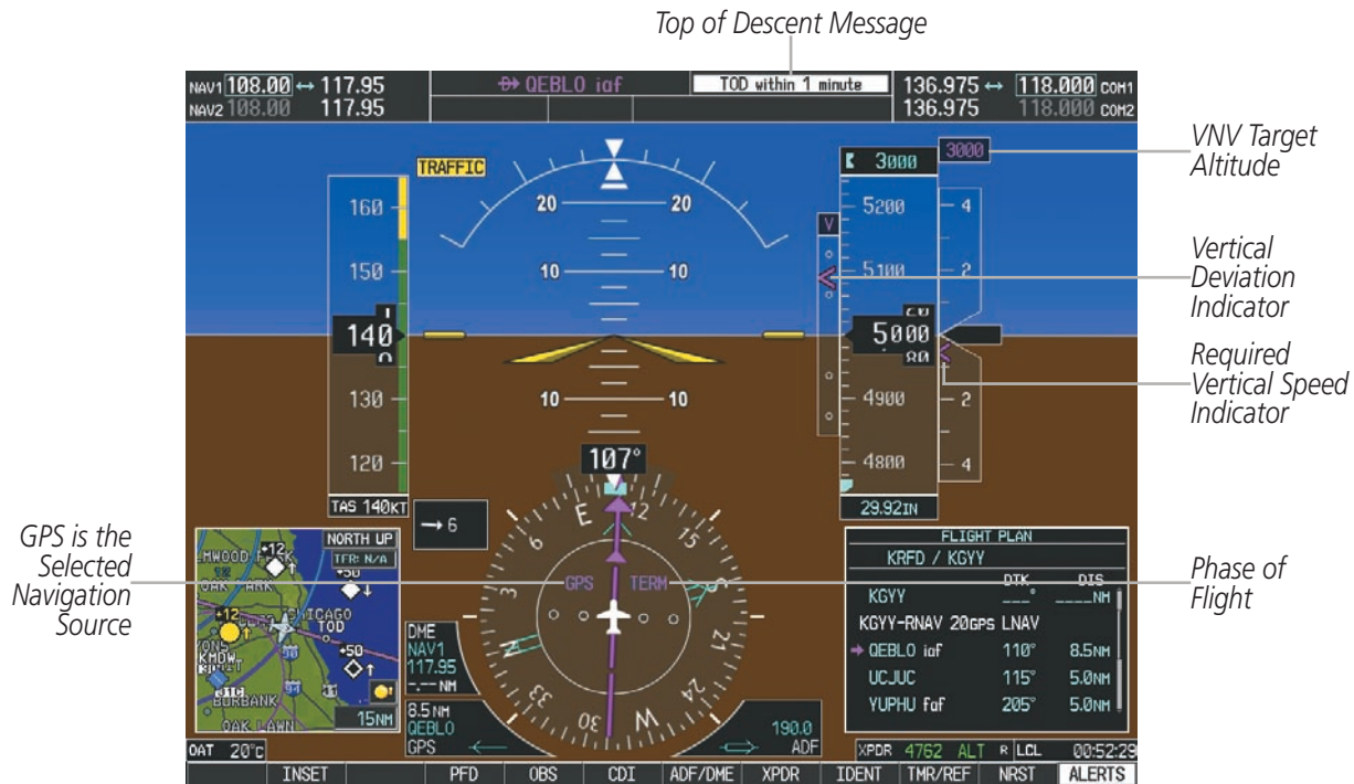
Figure 2-30 Vertical Navigation Indications (PFD)
