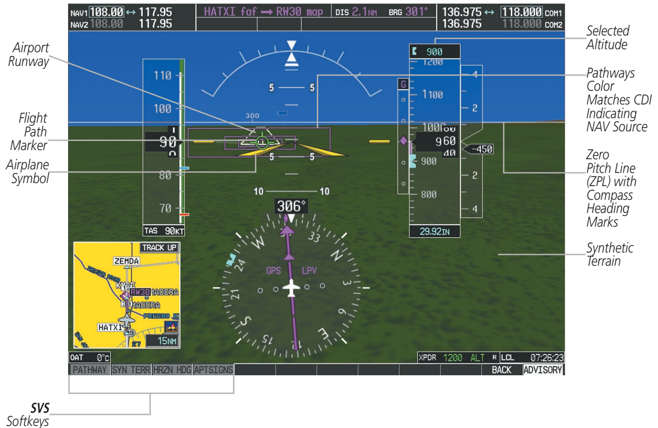
Figure 8-3 SVS on the Primary Flight Display
