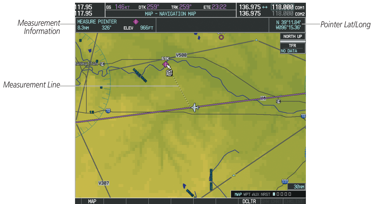
Figure 5-13 Navigation Map - Measuring Bearing and Distance
