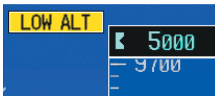
Figure 2-35 Low Altitude on GPS WAAS Approach
