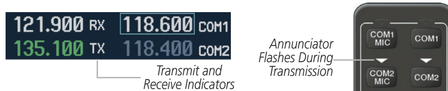
Figure 4-4 COM Radio Transmit and Receive Indications
