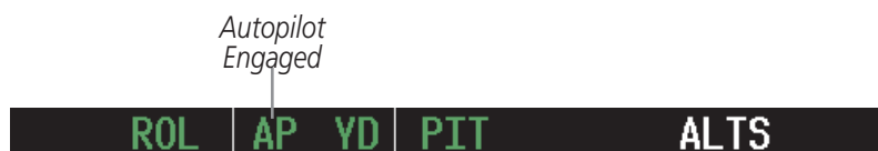
Figure 7-26 Autopilot and Yaw Damper Engaged
