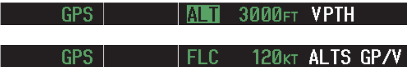
Figure 7-10 Vertical Path Tracking Armed Annunciations
