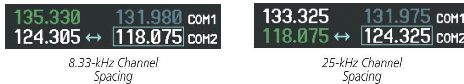
Figure 4-13 COM Channel Spacing
