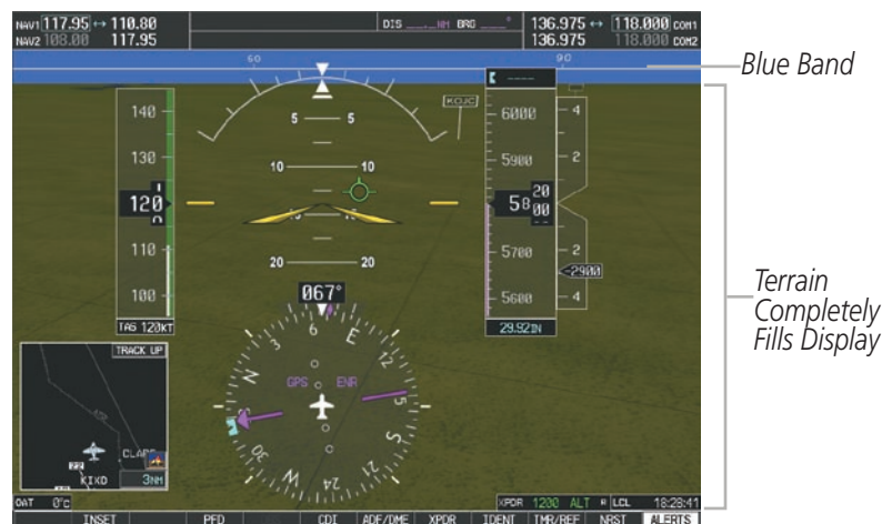
Figure 8-82 Blue Sky Bar with Full Display Terrain
