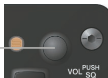
Figure 4-15 Overriding Automatic Squelch
