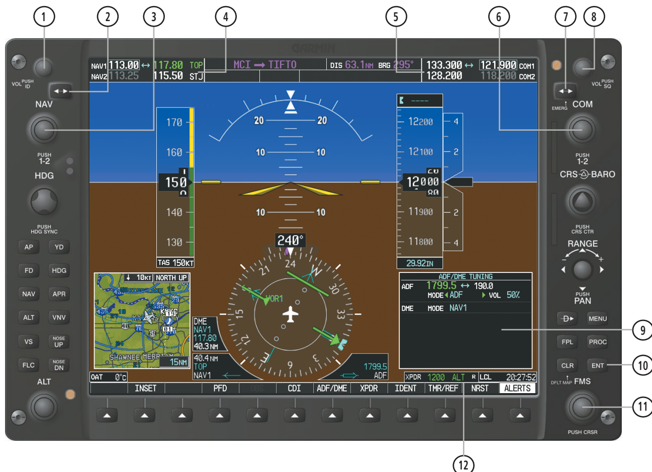
Figure 4-1 MFD/PFD Controls, NAV/COM Frequency Tuning Boxes, and ADF/DME Tuning Window (PFD Shown)
