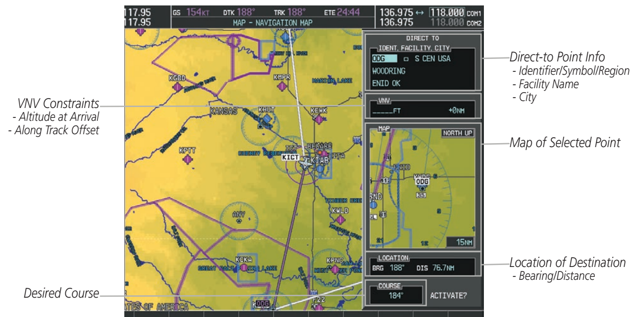
Figure 5-49 Direct-to Window - MFD
