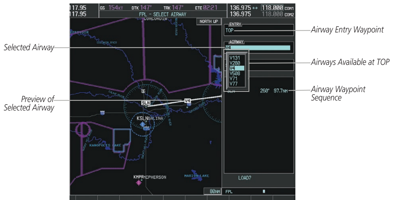
Figure 5-60 Select Airway Page - Selecting Airway
