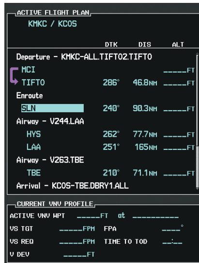
Figure 5-103 Begin Adding V4 to the Flight Plan
