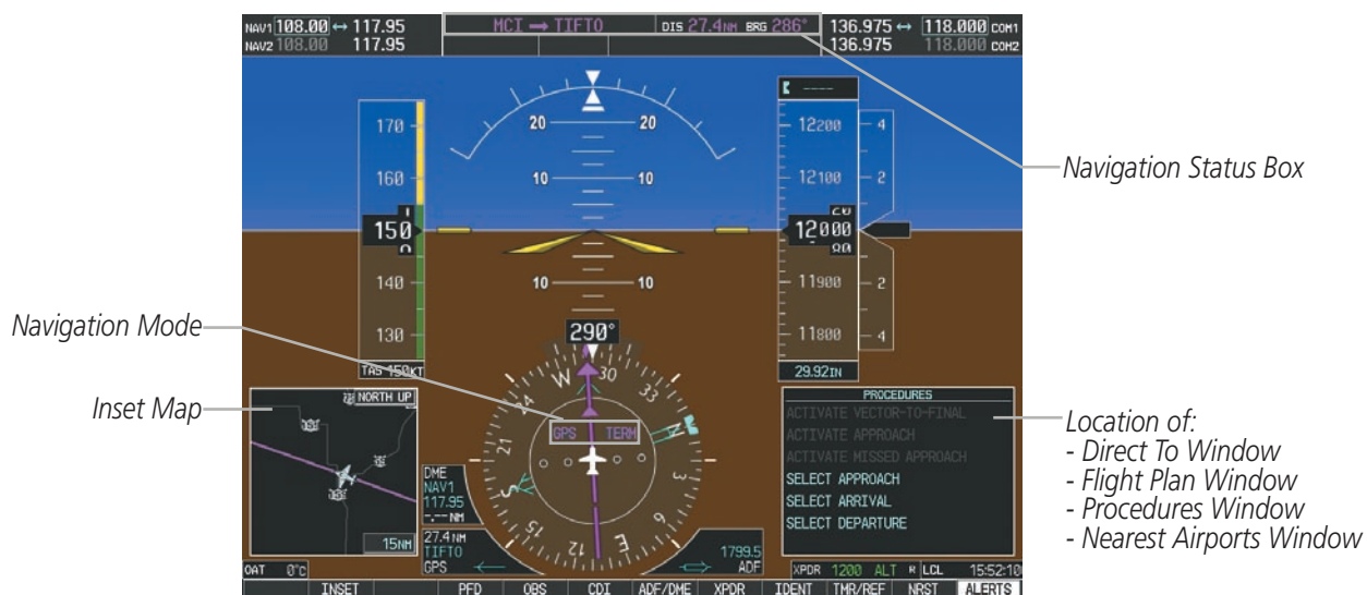
Figure 5-1 GPS Navigation Information on the PFD
