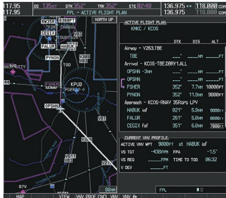
Figure 5-132 Tracking the OPSHN to FSHER Leg
