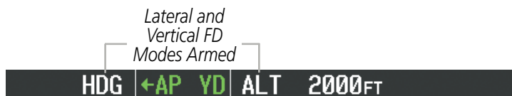
Figure 7-34 Lateral and Vertical Flight Director Modes Armed
