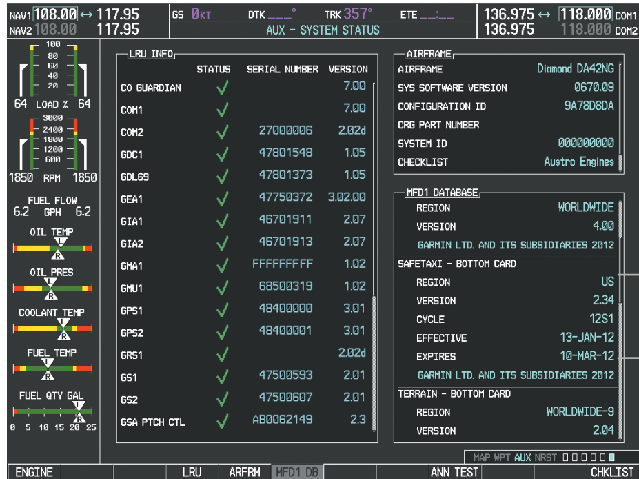
Figure 8-18 AUX – System Status Page, SafeTaxi Current Information
