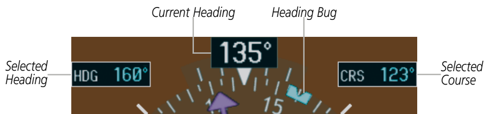
Figure 2-13 Heading and Course Indications (Magnetic)
