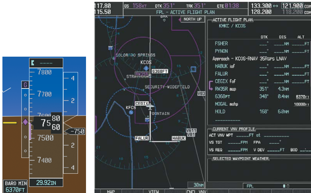
Figure 5-142 Descending to the Missed Approach Point
