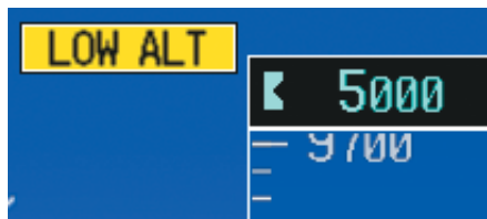
Figure 2-35 Low Altitude on GPS SBAS Approach
