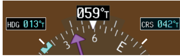
Figure 2-14 Heading and Course Indications (True)
