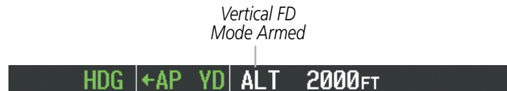
Figure 7-36 Vertical Flight Director Mode Armed
