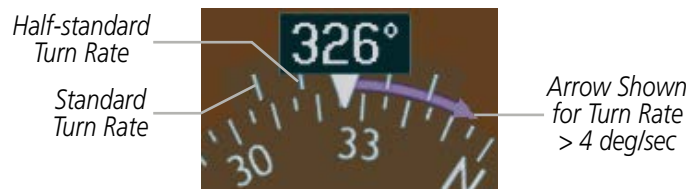
Figure 2-16 Turn Rate Indicator and Trend Vector
