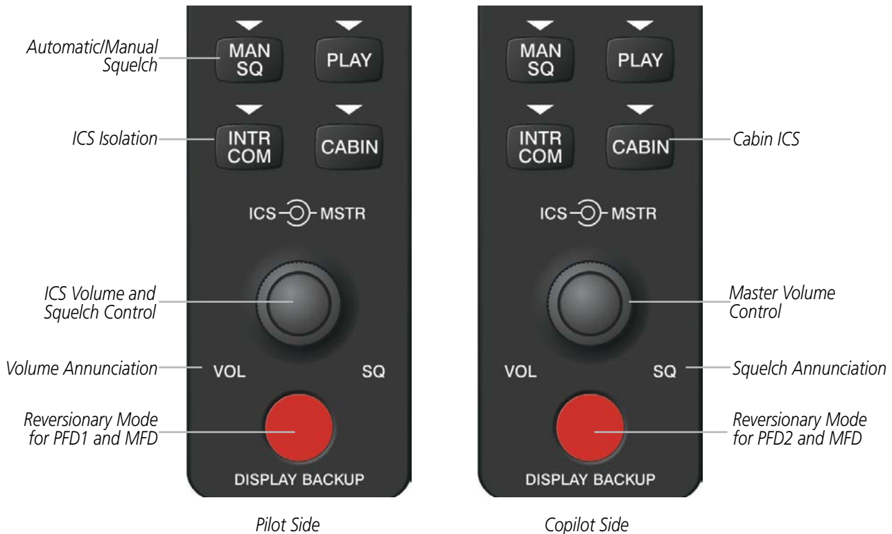
Figure 4-61 Audio Panel Controls
