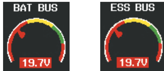
Figure 3-25 Battery and Essential Bus Low Voltage
