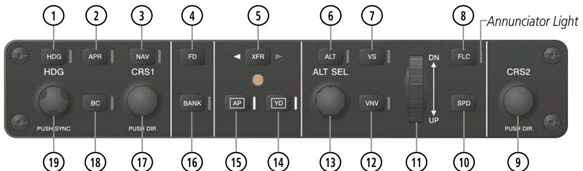
Figure 7-1 GMC 710 AFCS Control Unit
