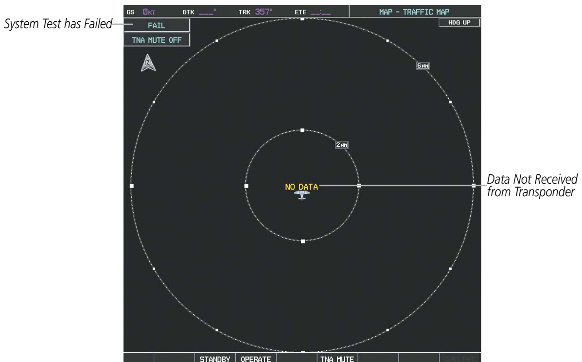
Figure 6-169 TIS Power-up Test Failure
