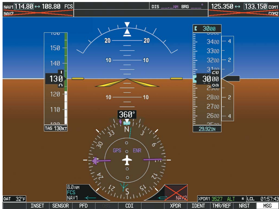
Figure 4-66 PFD1 Display after PFD2 Failure
