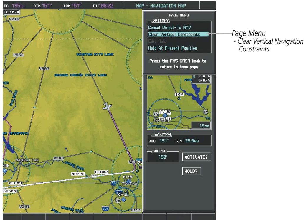
Figure 5-55 Direct-to Window - Clearing Vertical Constraints
