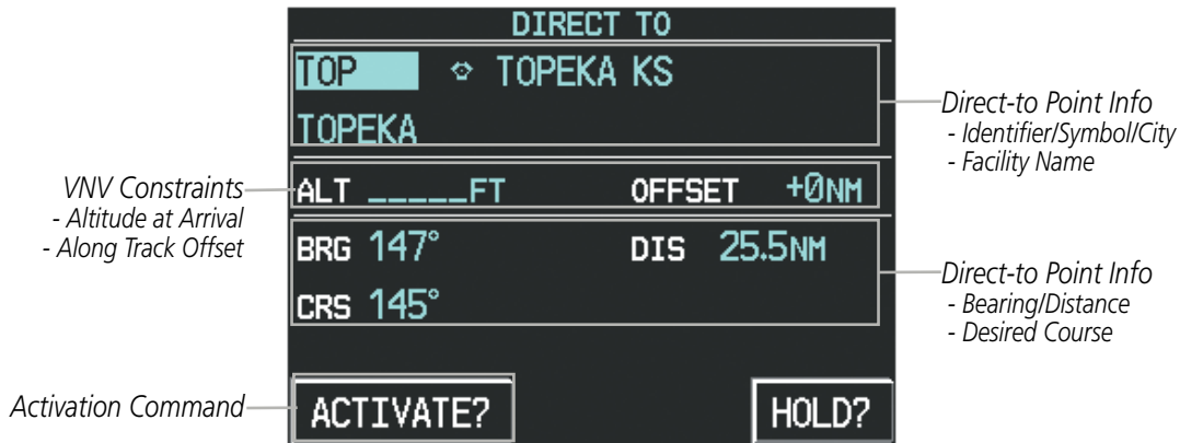
Figure 5-52 Direct-to Window - PFD
