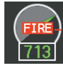
Figure 3-24 Engine Fire Indication
