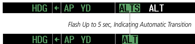
Figure 7-8 Automatic Mode Transitions During Altitude Capture
