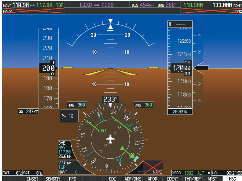
Figure 4-69 PFD1 Display after PFD2 Failure with HSDB Switch in REV Mode
