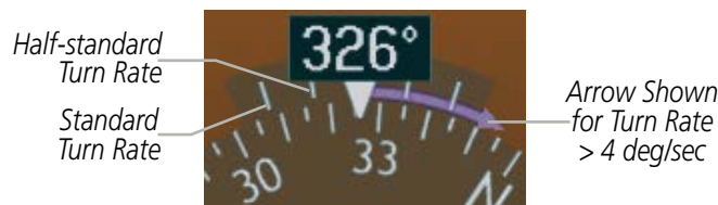
Figure 2-23 Turn Rate Indicator and Trend Vector
