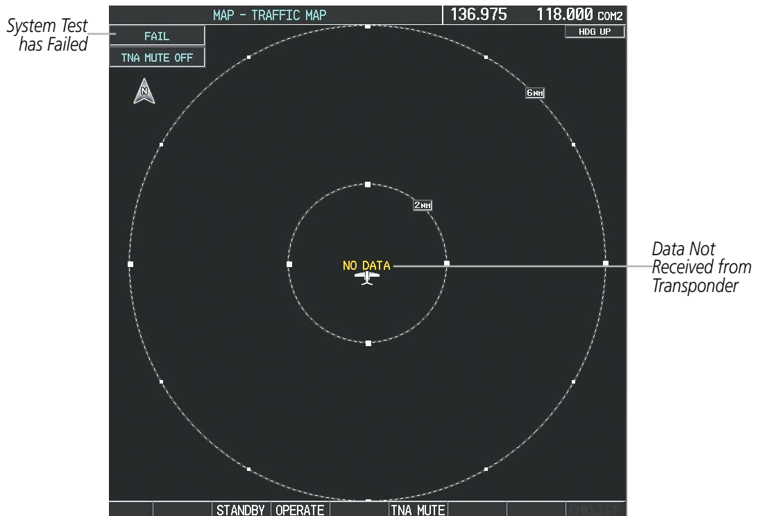
Figure 6-161 TIS Power-up Test Failure
