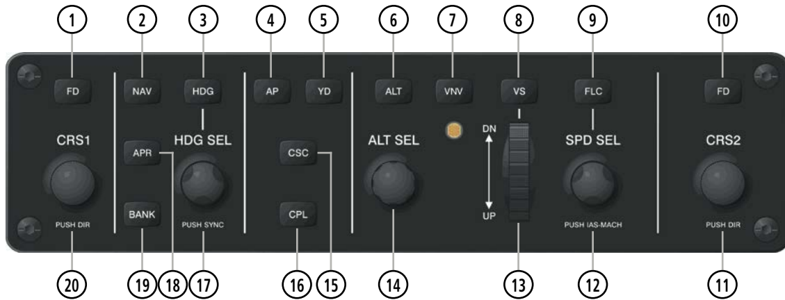
Figure 7-1 GMC 715 AFCS Control Unit
