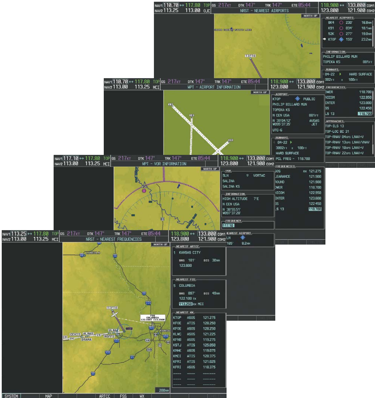
Figure 4-37 NRST – Nearest Frequencies, WPT – VOR Information, WPT – Airport Information, and NRST – Nearest Airports Pages
