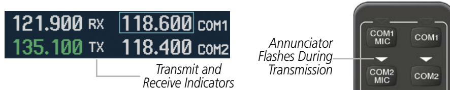
Figure 4-4 COM Radio Transmit and Receive Indications
