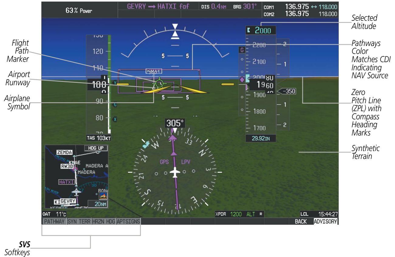
Figure 8-3 SVS on the Primary Flight Display
