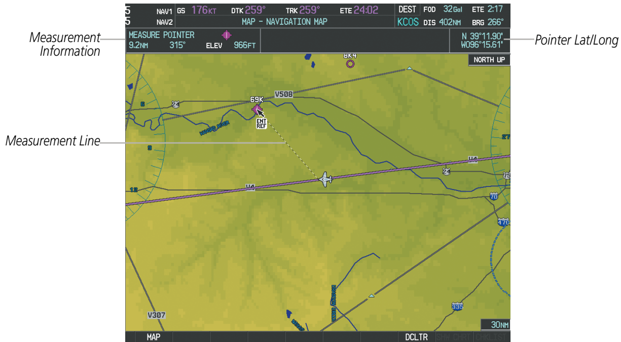
Figure 5-13 Navigation Map - Measuring Bearing and Distance
