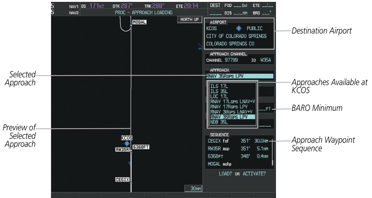
Figure 5-75 Approach Loading Page - Selecting the Approach
