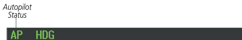
Figure 7-49 Autopilot Engaged (Perspective™ AFCS Status Box)
