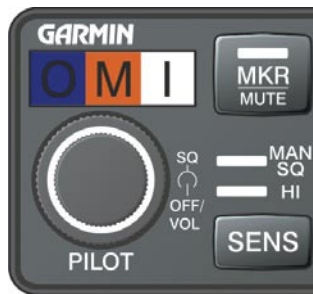
Figure 4-32 Marker Beacon Keys and Annunciator Lights
