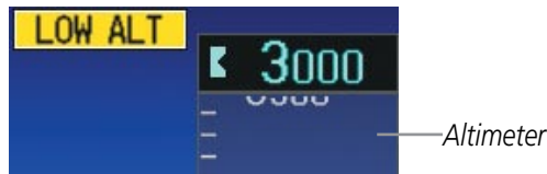
Figure 2-38 Low Altitude on GPS SBAS Approach
