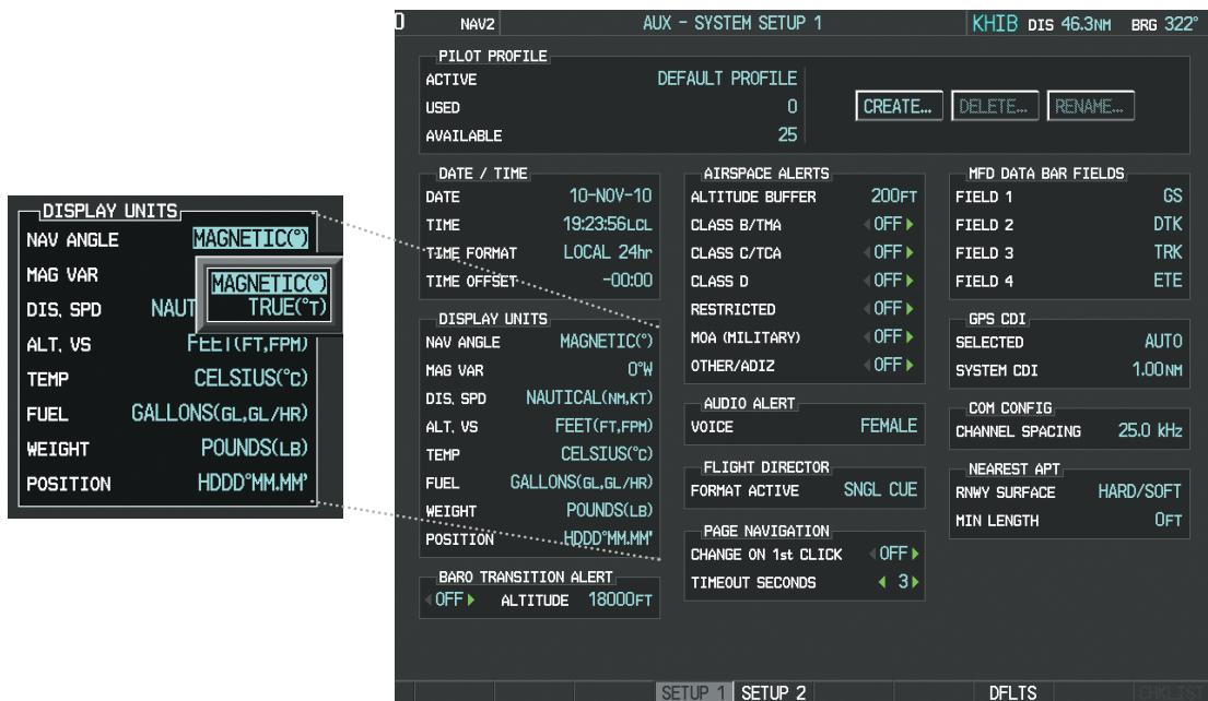
Figure 2-17 Navigation Angle Settings (AUX - System Setup Page)
