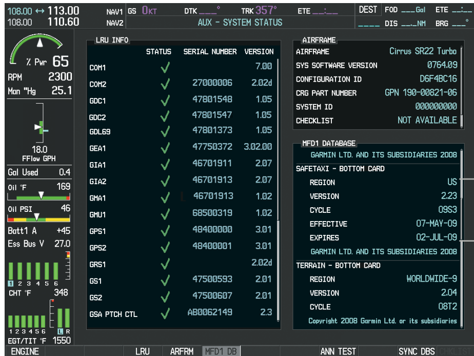
Figure 8-23 AUX – System Status Page, SafeTaxi Current Information
