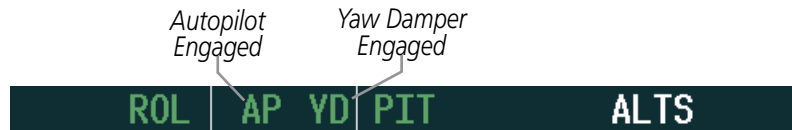
Figure 7-27 Autopilot and Yaw Damper Engaged
