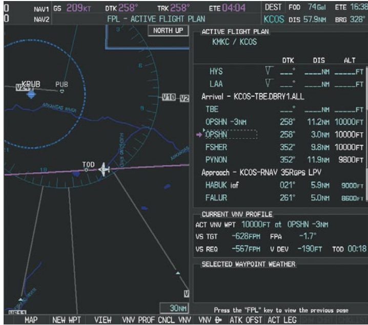
Figure 5-132 Approaching Top of Descent (TOD)
