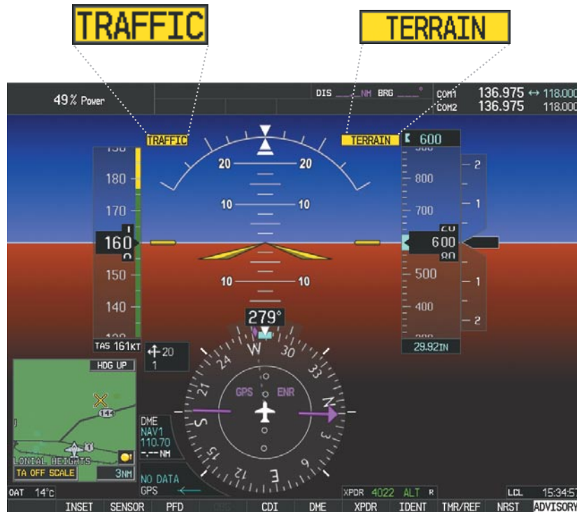
Figure 2-36 Traffic and Example TAWS Annunciations
