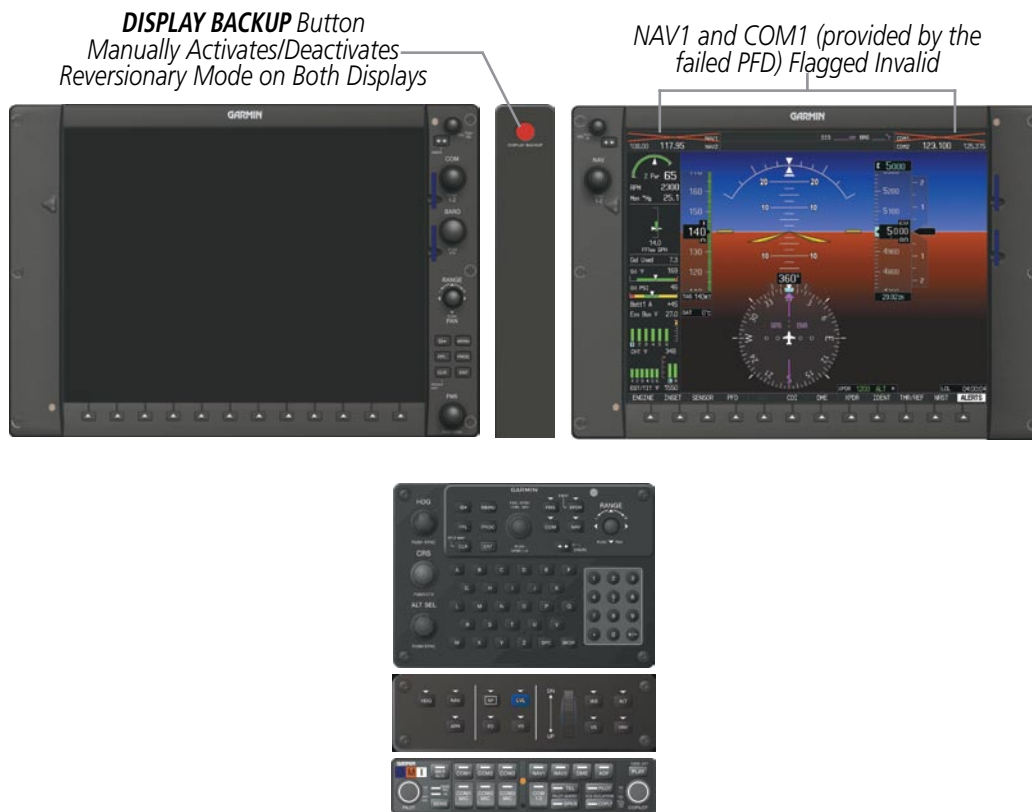
Figure 1-18 Reversionary Mode (Failed PFD)
