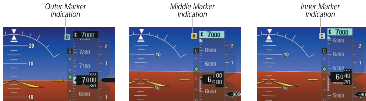
Figure 4-31 Marker Beacon Annunciations on the PFD
