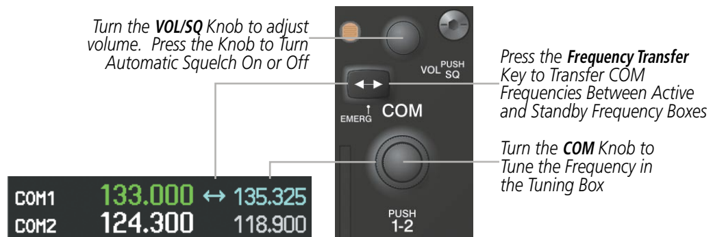
Figure 4-8 COM Frequency Tuning
