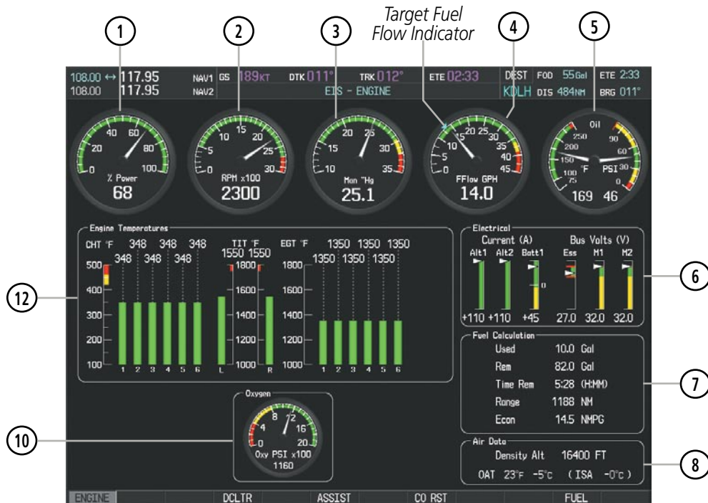
Figure 3-8 Engine Page (SR22TN) with Oxygen
