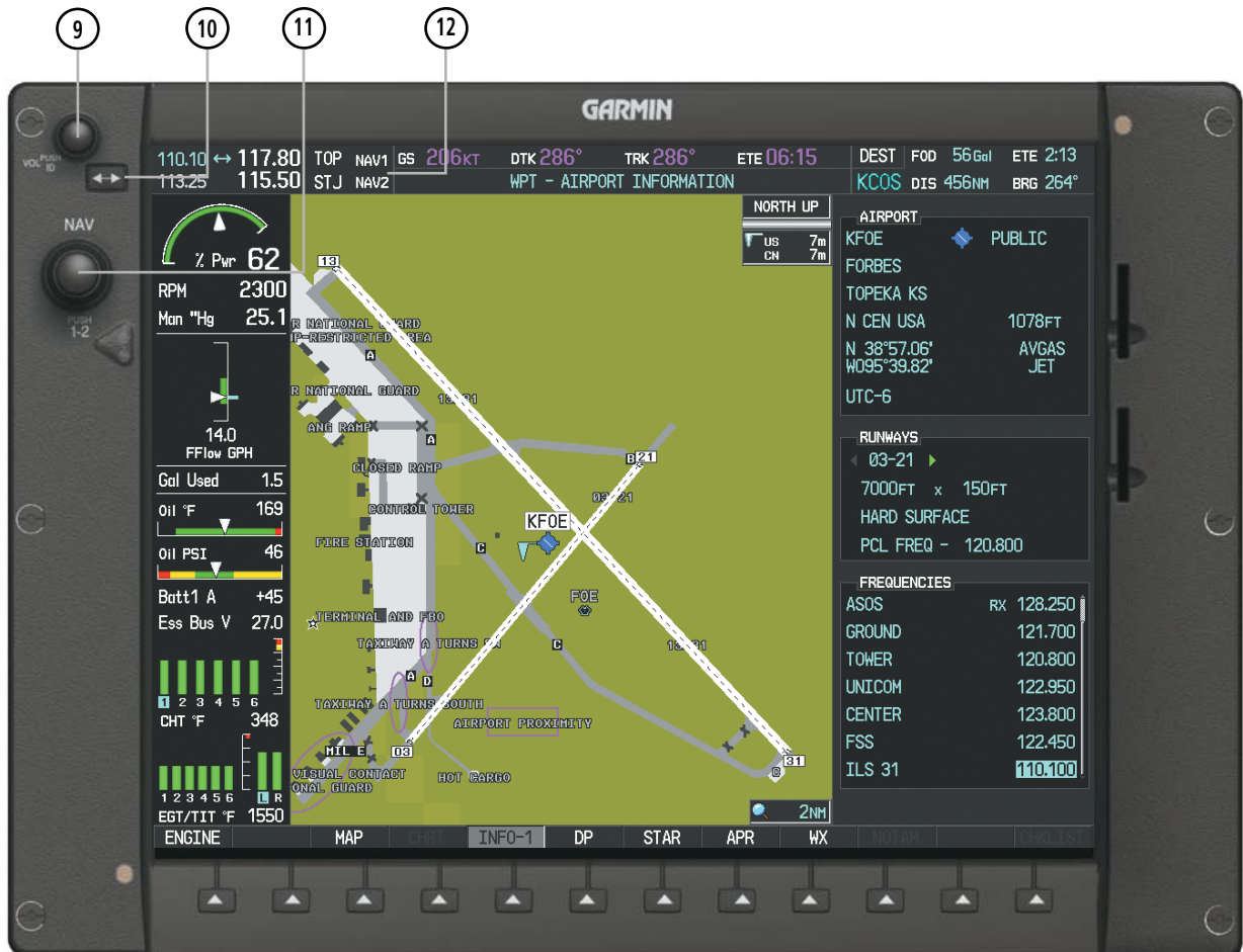
Figure 4-2 MFD Controls and NAV Frequency Tuning Boxes
