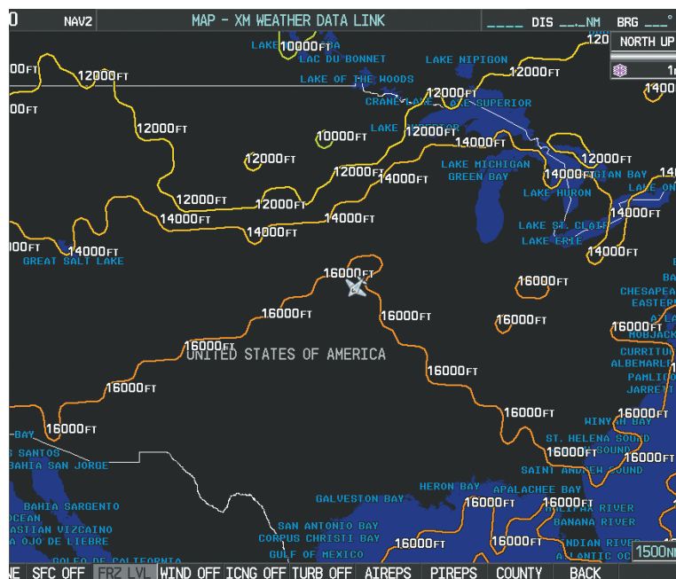
Figure 6-30 Freezing Level Data
