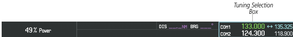
Figure 4-5 Frequency Tuning with the Control Unit
