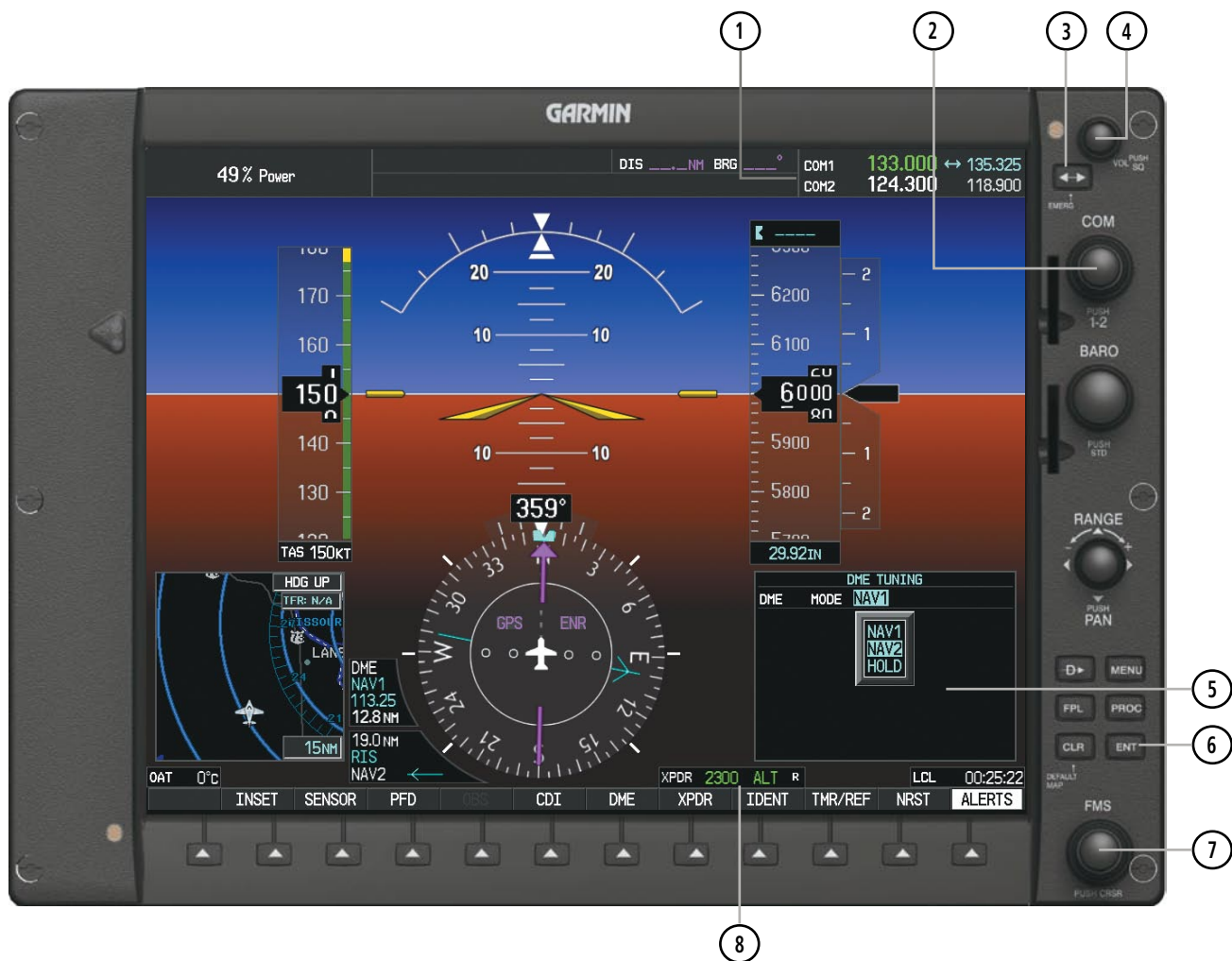
Figure 4-1 PFD Controls, COM Frequency Tuning Boxes, Transponder Code, and DME Tuning Window
