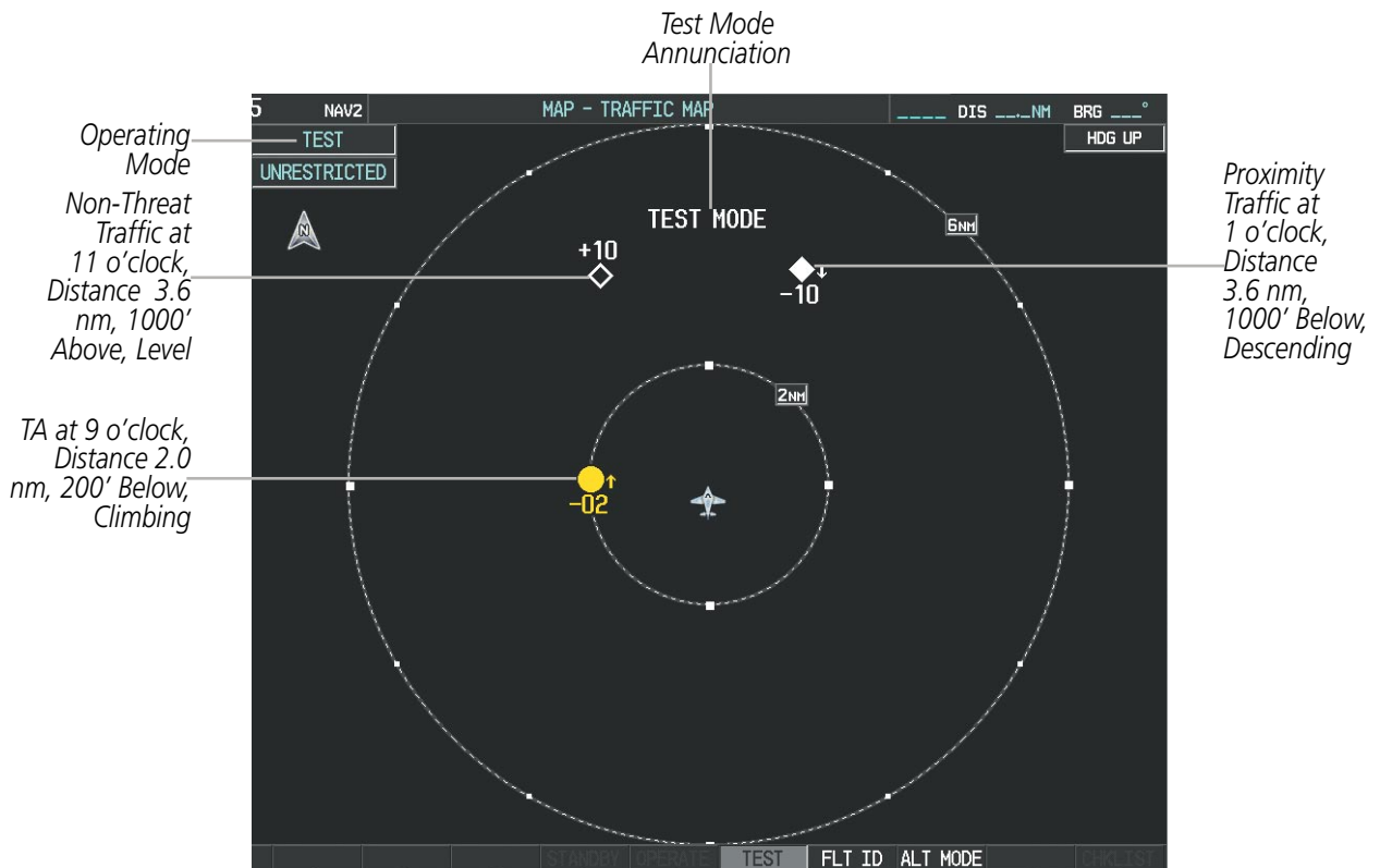
Figure 6-89 System Test in Progress with Test Pattern
