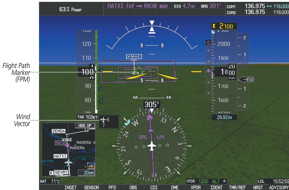
Figure 8-7 Flight Path Marker and Pathways
