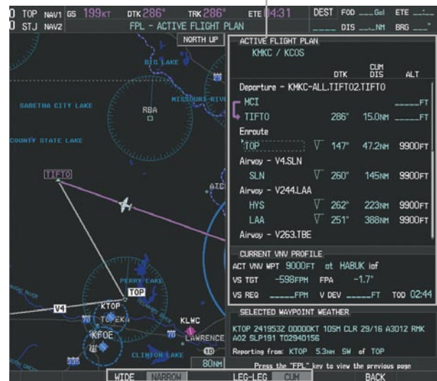
Active Flight Plan Cumulative Distance
