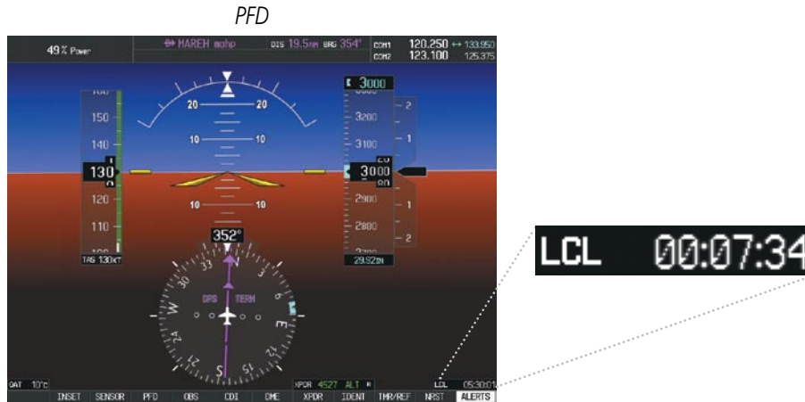
Figure 1-33 System Time (Local 24-hr Format)
