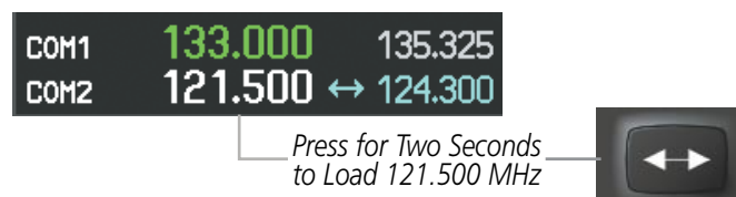
Figure 4-11 Quickly Tuning 121.500 MHz
