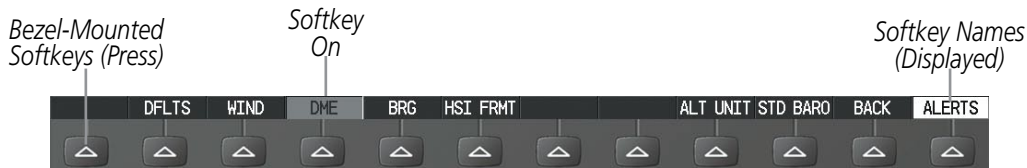
Figure 1-6 Softkeys (Second-Level PFD Configuration)
