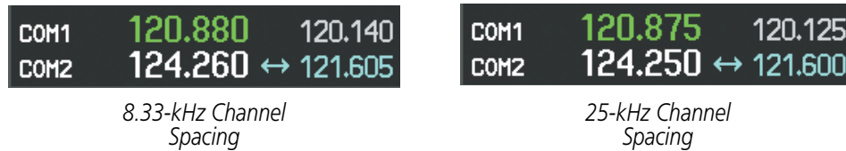
Figure 4-17 COM Channel Spacing
