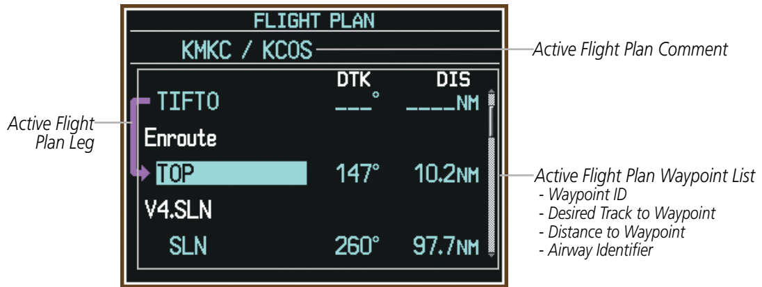
Figure 5-58 Active Flight Plan Window on PFD
