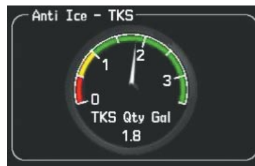
Figure 3-13 TKS NH System Fluid Quantity Gauge
