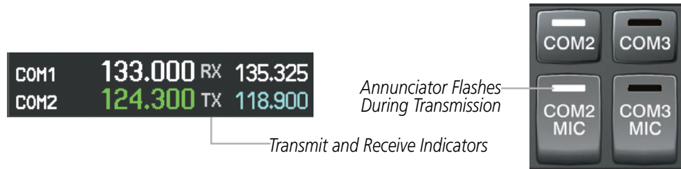
Figure 4-7 COM Radio Transmit and Receive Indications
