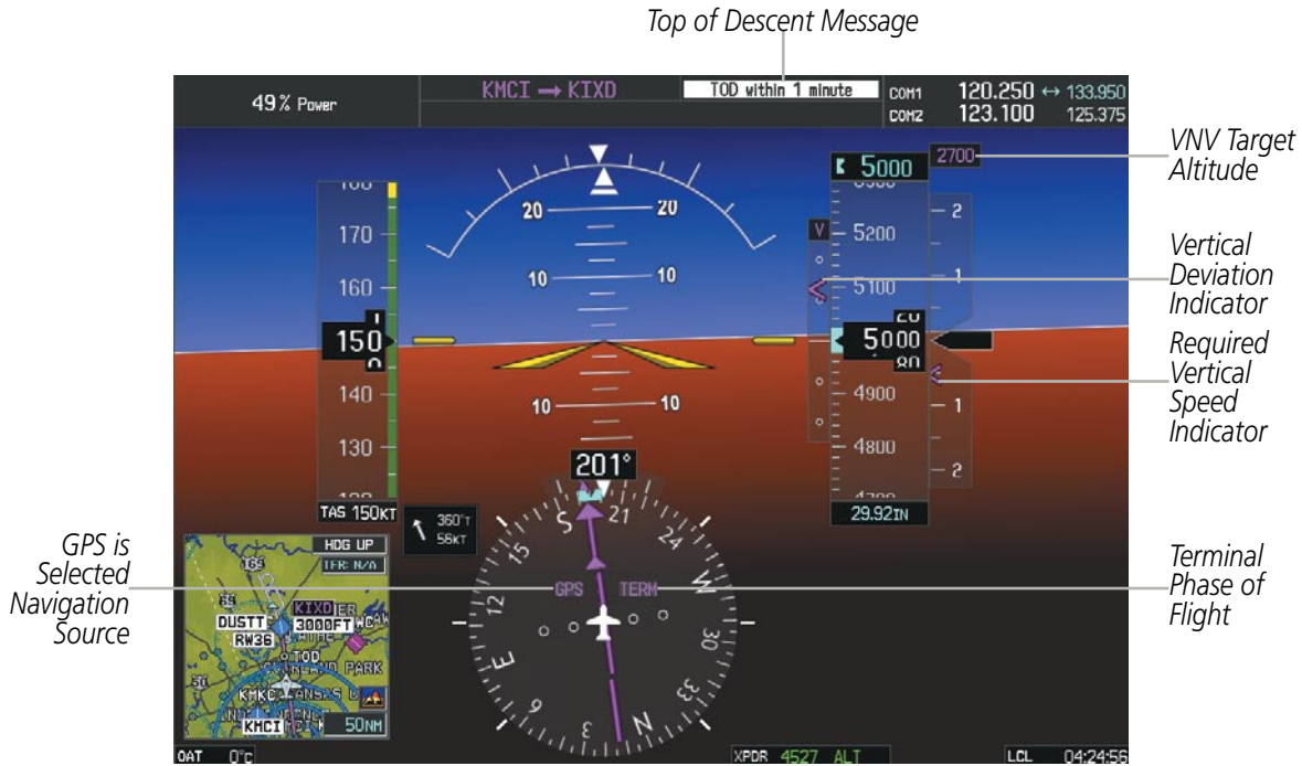
Figure 2-32 Vertical Navigation Indications (PFD)
