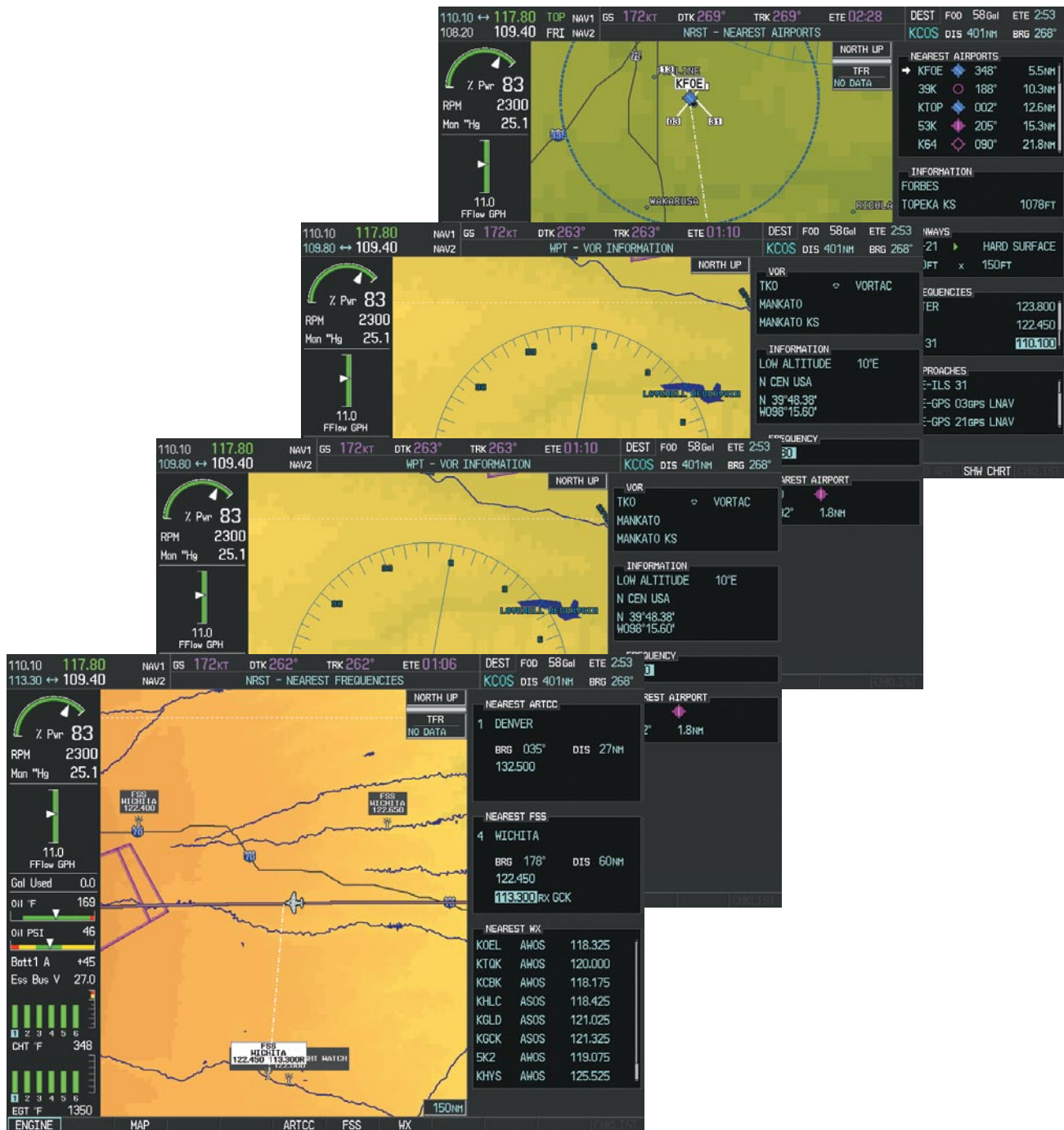
Figure 4-30 NRST – Nearest Frequencies, WPT – VOR Information, WPT – Airport Information, and NRST – Nearest Airports Pages
