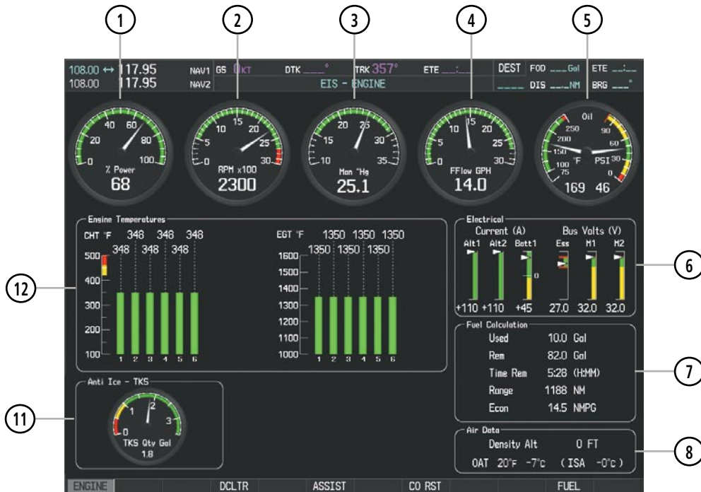
Figure 3-6 Engine Page (SR22) with TKS NH Anti-Ice Option
