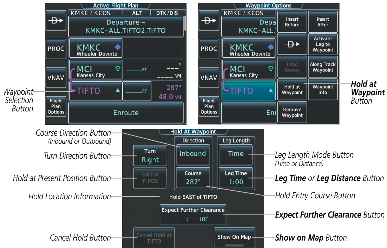
Figure 5-122 Creating a User Defined Holding Pattern at an Active Flight Plan Waypoint
