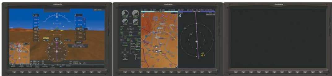
Figure 1-28 Automatic Reversionary Mode - PFD2 Failure
