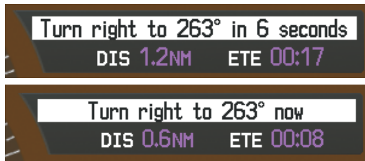
Figure 5-163 Turn to Intercept V244
