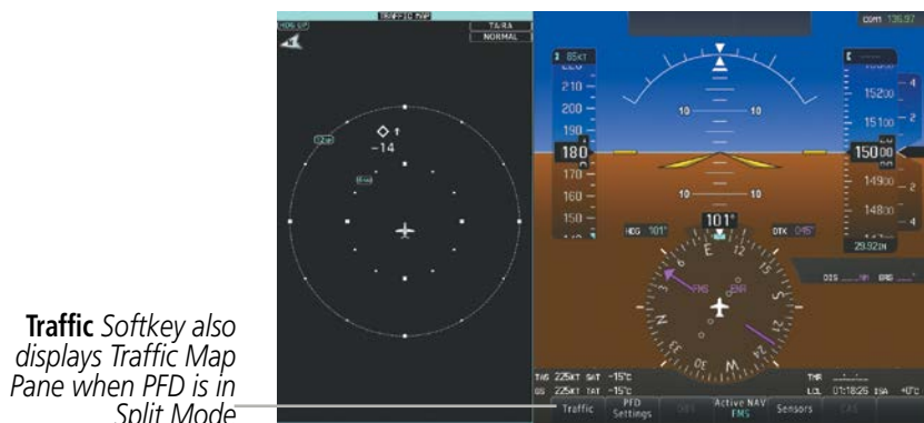
Figure 6-79 Using the Traffic Softkey to show Traffic Map Pane (PFD in Split Mode)
