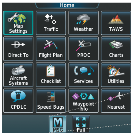
Figure A-7 System Messages Annunciation (Touchscreen Controller)
