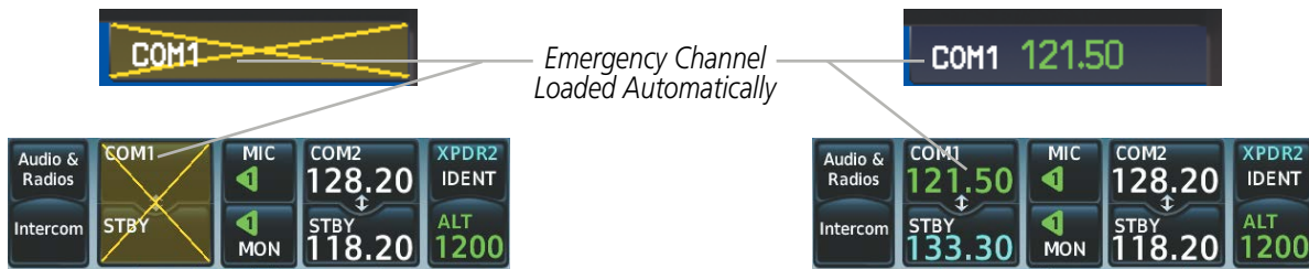
Figure 4-83 COM Tuning Failure
