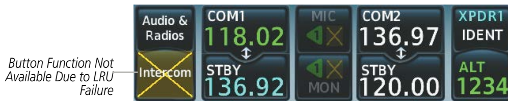
Figure 1-20 Failed Buttons on Touchscreen Controller
