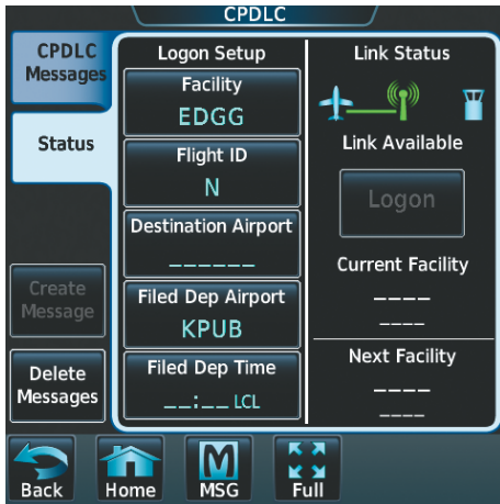
Figure 4-63 CPDLC Log-On Facility Set
