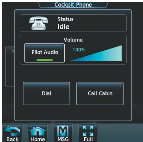
Figure 8-61 Cockpit Telephone Status
