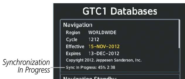
Figure B-7 Avionics Status Screen, Database Information Window, Navigation Database Sync in Progress
