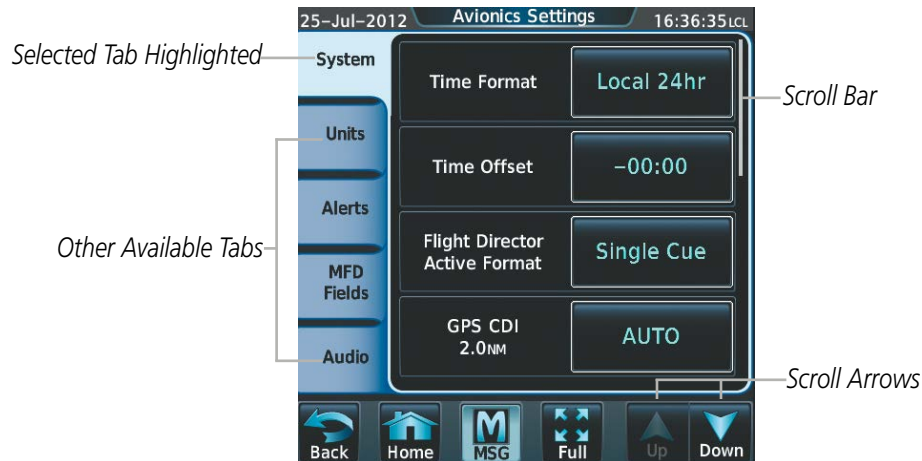
Figure 1-16 Touchscreen Controller with Tabs and Scroll Arrows
