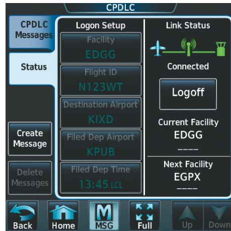
Figure 4-72 System is Connected and Active
