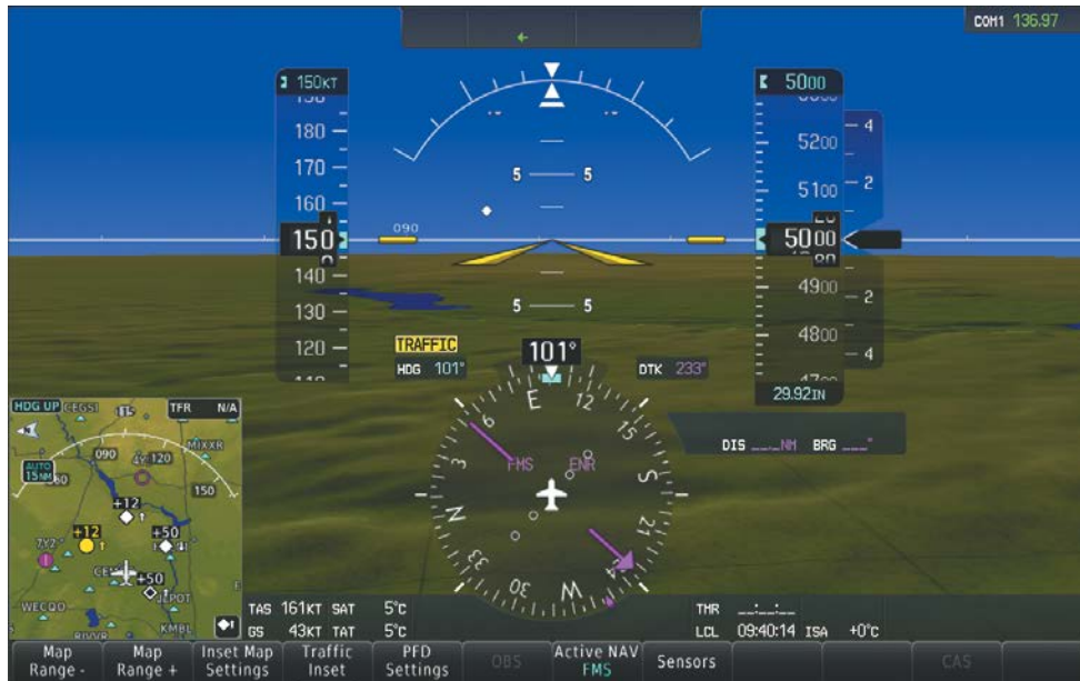
Figure 2-32 Synthetic Vision Imagery
