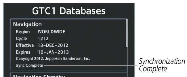
Figure B-8 Avionics Status Screen, Database Information Window, Navigation Database Sync Complete
