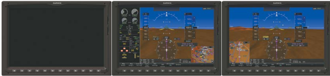
Figure 1-26 Automatic Reversionary Mode - PFD1 Failure
