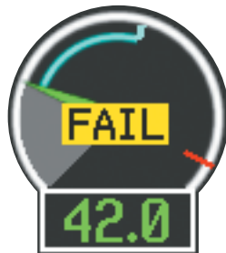
Figure 3-24 Engine Failure Indication
