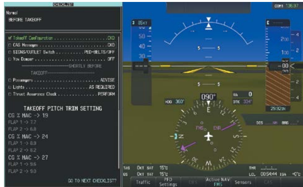
Figure 8-152 First Checklist Item Completed and Checked
