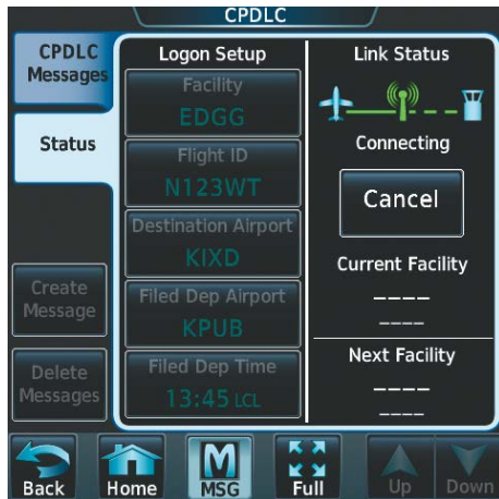
Figure 4-71 CPDLC Connecting to ATC Facility
