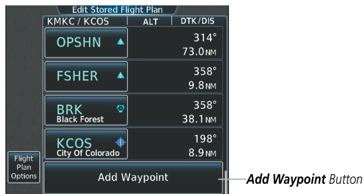
Figure 5-88 Edit Stored Flight Plan Screen - Adding a Waypoint to the end of the Flight Plan
