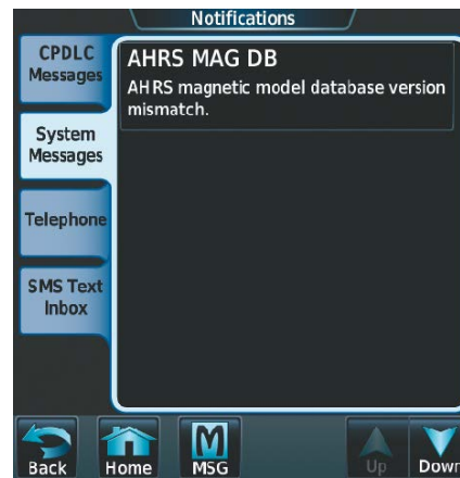
Figure B-16 Database Mismatch Message is Annunciated Before Second GRS is Updated
