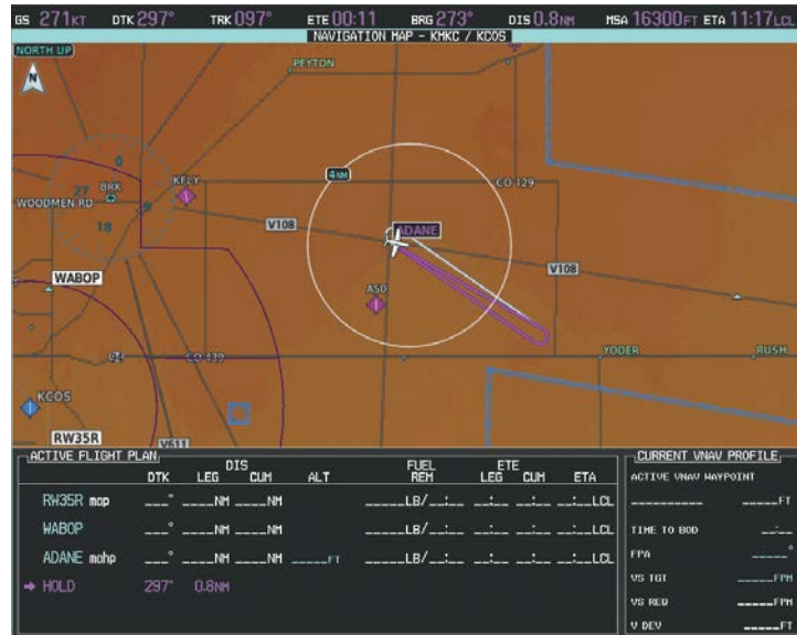
Figure 5-194 Establishing the Holding Pattern
