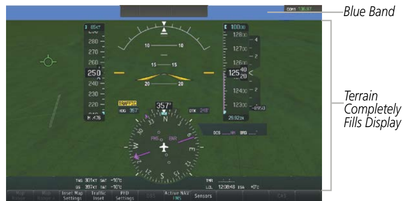
Figure 2-59 Blue Sky Bar with Full Display Terrain
