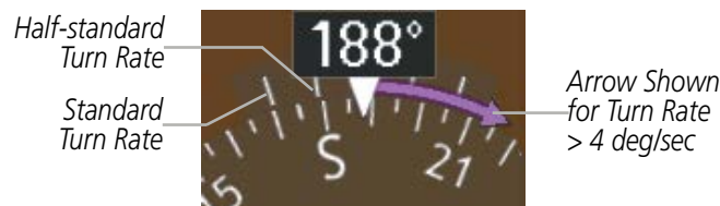
Figure 2-21 Turn Rate Indicator and Trend Vector
