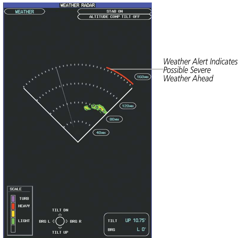
Figure 6-53 Weather Alerts on the Weather Radar Pane
