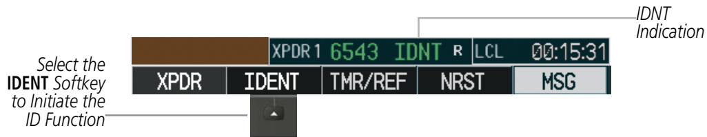
Figure 4-47 IDENT Softkey and Indication
