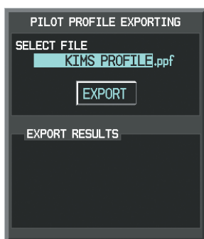
Pilot Profile Exporting Window, Enter a Name to Use for Exported Profile
