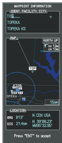
Figure 5-116 Entering V4 Entry Point
