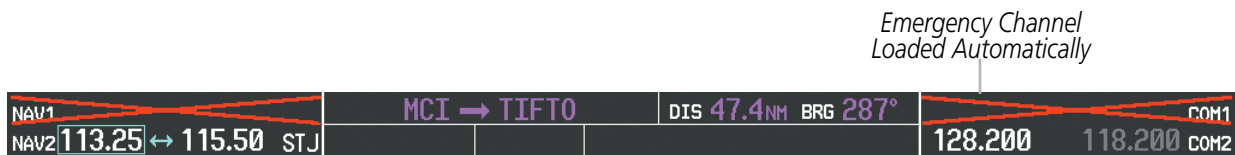
Figure 4-66 Frequency Section of PFD2 Display after PFD1 Failure
