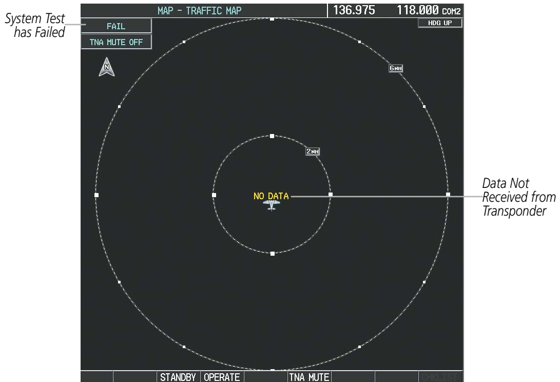
Figure 6-161 TIS Power-up Test Failure
