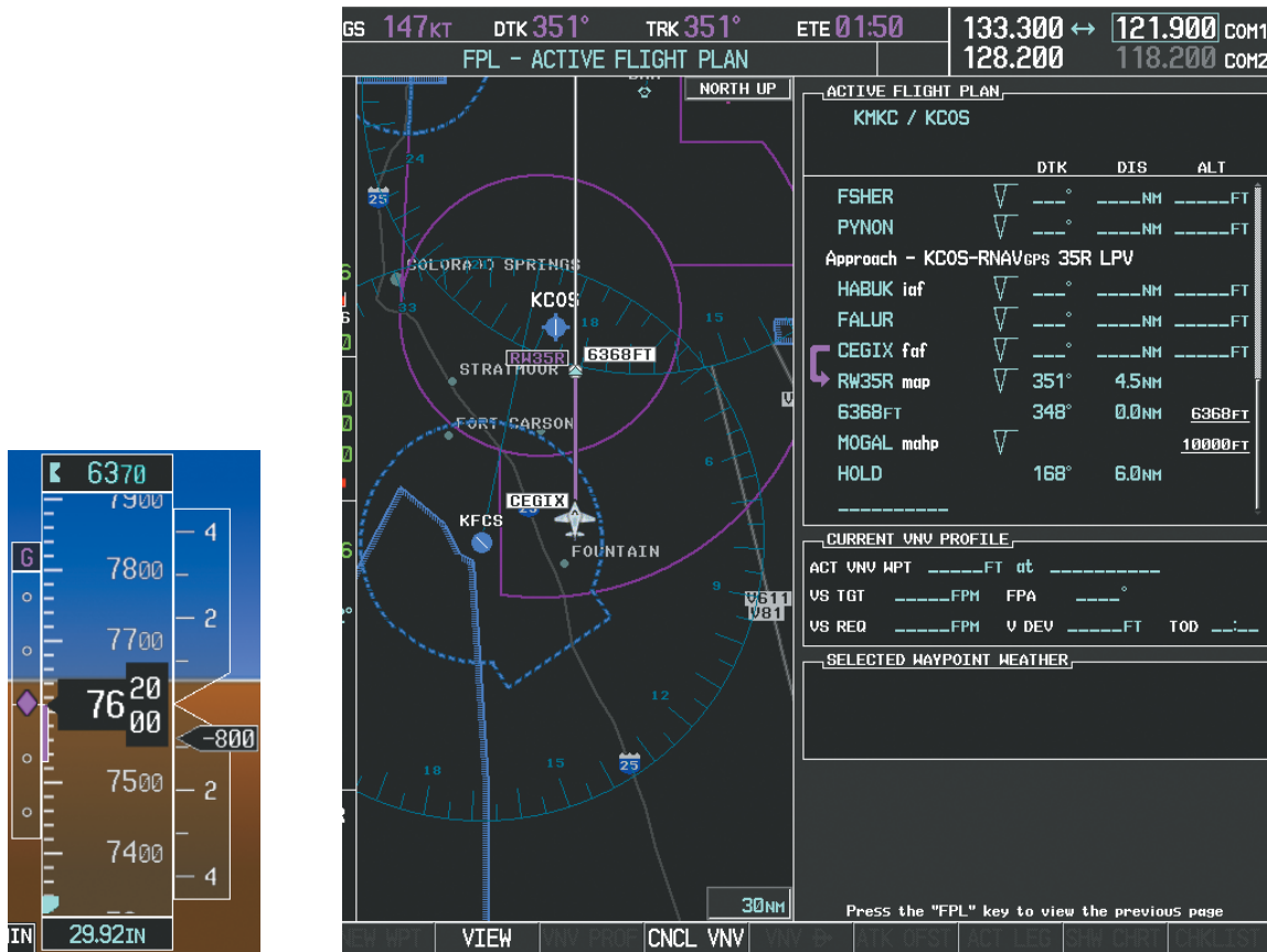
Figure 5-150 Descending to the Missed Approach Point
