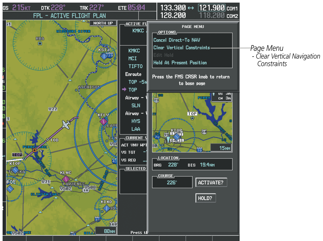
Figure 5-55 Direct-to Window - Clearing Vertical Constraints
