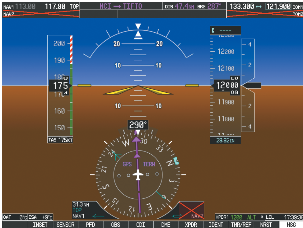
Figure 4-67 PFD1 Display after PFD2 Failure
