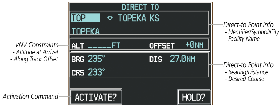
Figure 5-52 Direct-to Window - PFD
