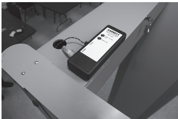
(Above) Wireless Synchronization Module mounted externally.
