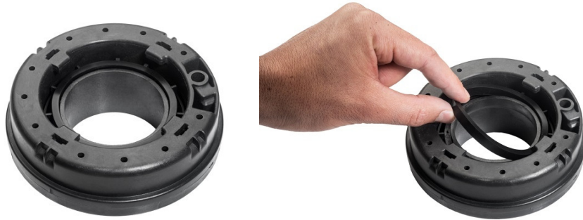
Figure 35: Freightliner Extension-Tag installation
