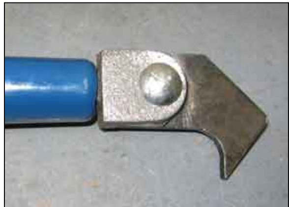
Gatekeeper Hook for cleaning out the saw cut
