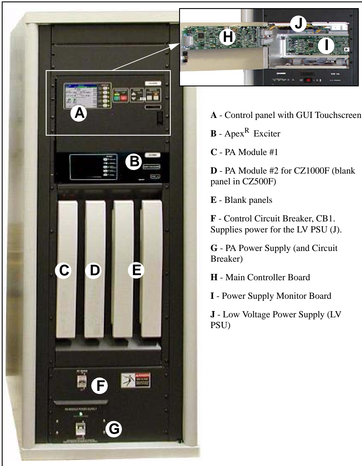
Figure 2-12 Component Locator, Cabinet Front View
