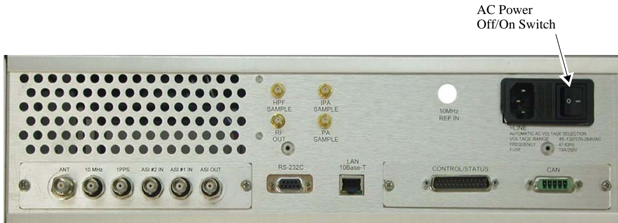
Figure 2-9 Exciter Inputs and Outputs
