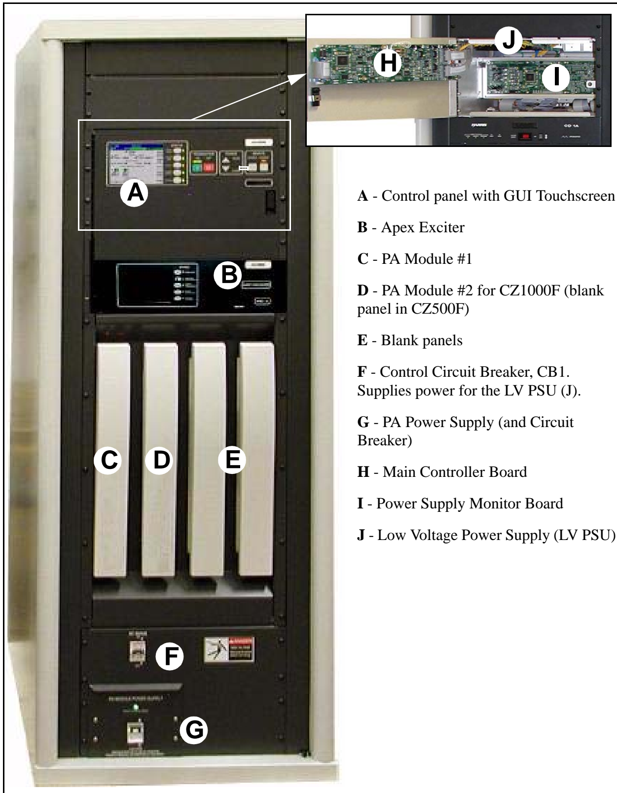
Figure 2-2 Component Locator, Cabinet Front View
