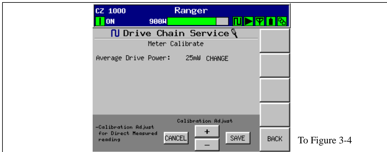
Figure 3-5 Drive Service Screen
