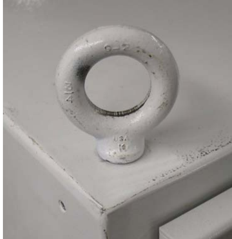
Figure 2-2 Lifting Eye Bolt On Top of Transmitter Cabinet
