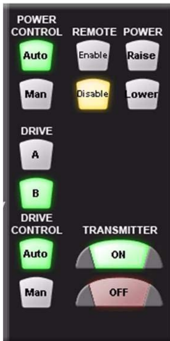
Figure 3-2 Transmitter Control Panel
