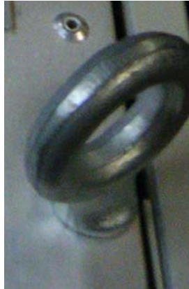
Figure 2-2 Lifting Eye Bolt On Top of Transmitter Cabinet
