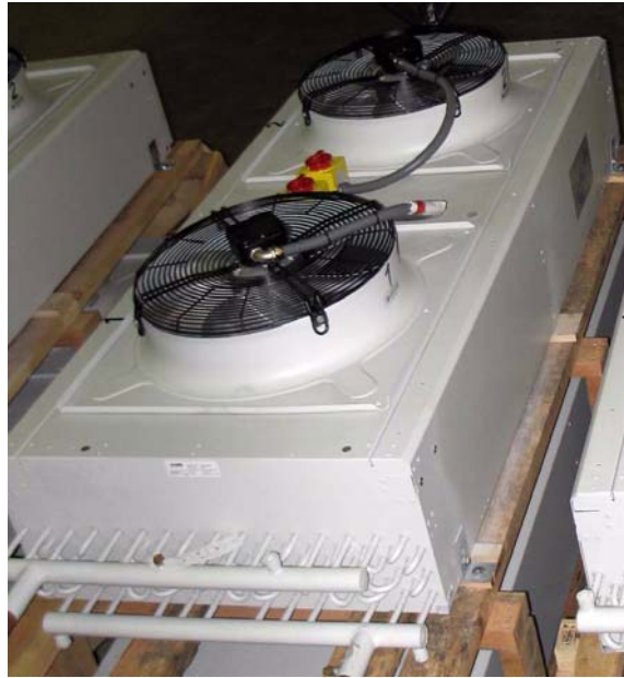
Figure 1-11 Heat Exchanger (before installation)
