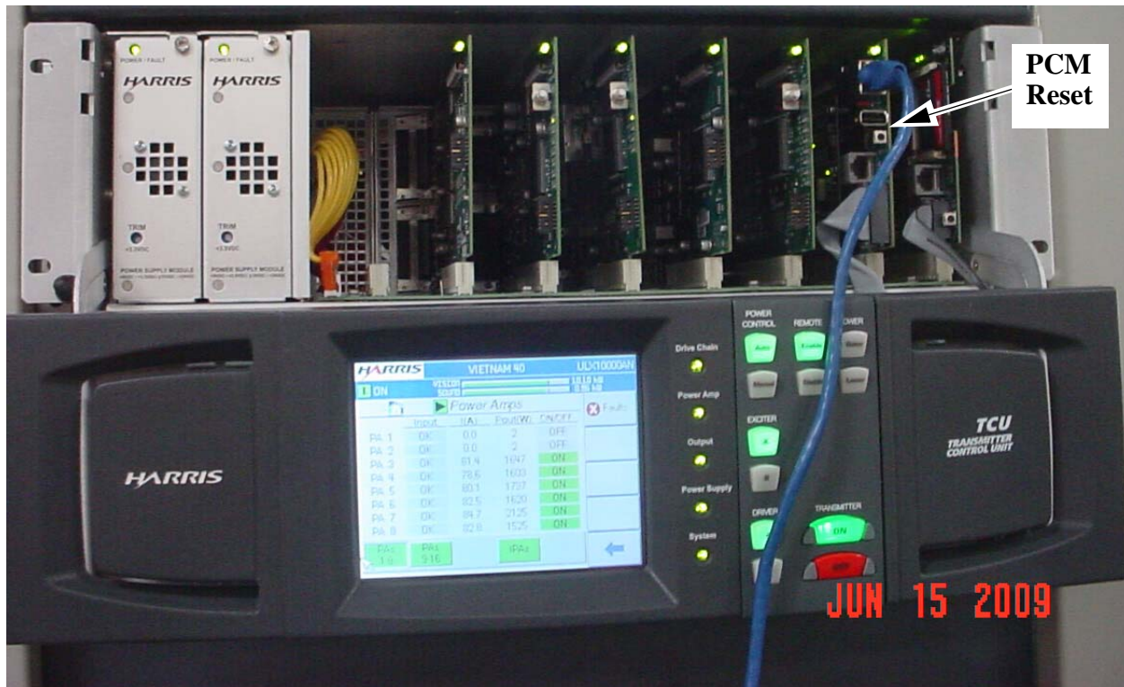
Figure 2-2 TCU Front Panel Lowered
