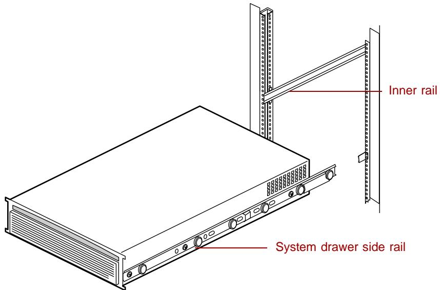
4 Push the system drawer evenly into the cabinet until the latches on the system drawer side rails lock.
