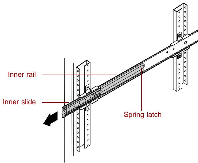
3 Lift the system drawer to the same height as the inner rails, then align the system drawer side rails with the inner rails.
