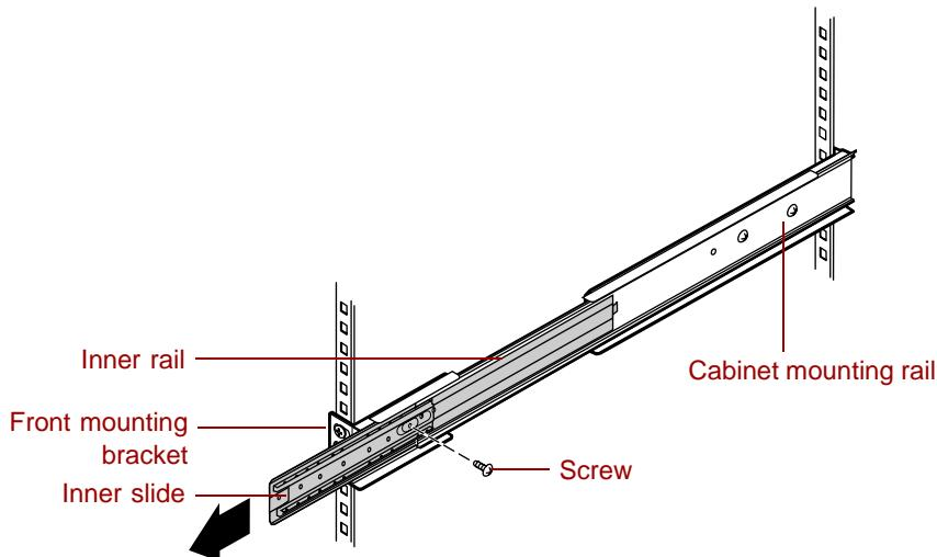
**4** Attach the front of the cabinet mounting rail to the front mounting bracket using a screw from the accessory kit.
