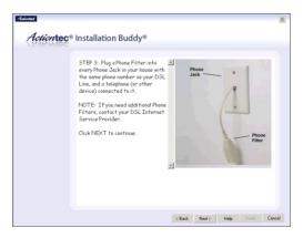
**5.** Plug the ends of the phone lines disconnected in step 2 into the phone filters plugged into phone jacks. Click **Next**.
