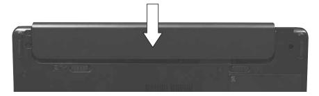
**4** Slide the battery lock to the locked position.
