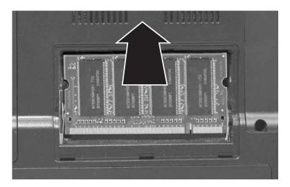
11 Hold the new or replacement module at a 30-degree angle and press it into the empty memory slot. This module is keyed so it can only be inserted in one direction. If the module does not fit, make sure that the notch in the module lines up with the tab in the memory bay.
