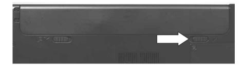
5 Slide the battery release latch, then slide the battery out of the notebook.
