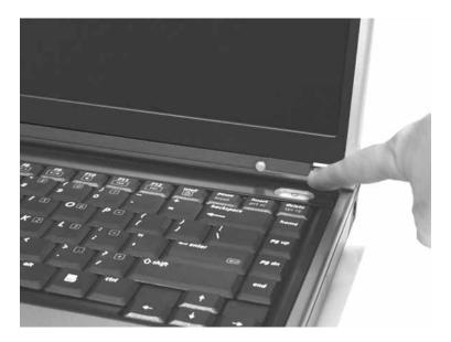
The power button is preset to On/Off mode. However, you can also set it to function in Standby/Resume mode.
