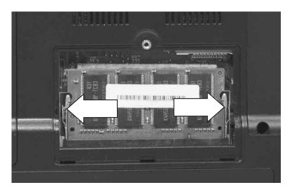
**10** Pull the memory module out of the slot.
