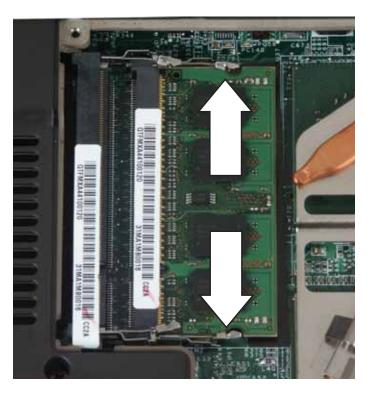
**9** Pull the memory module out of the slot.
