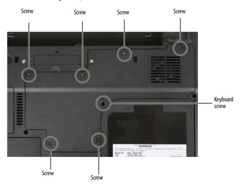
7 Use the thumb notch to lift the memory bay cover, then remove it. Be careful not to break off the tabs located on the end of the cover opposite of the thumb notch.
