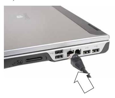
2 Insert the other end of the network cable into a cable modem, DSL modem, or Ethernet network jack.
