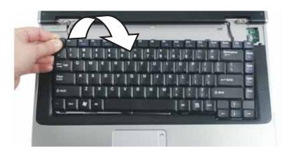
www.gateway.com Replacing the keyboard
