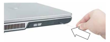
12 Carefully slide the drive out of the drive bay.
