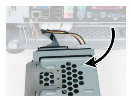
Disconnect the drive cable and power cable from the hard drive.
