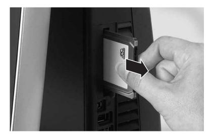
**3** Eject the PC Card by pressing the eject button again.
