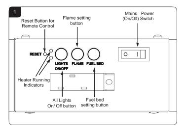
Note: The remote control will lose the memory for all function settings when the switch is set to the Off Position.
