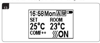
If the heater is on in the current period, pressing the button will turn the heater off.
