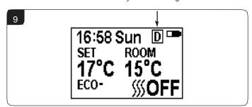
2b.21 Hold the button for 6 seconds to enter the daily heating setting.
