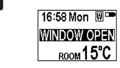
2b.45 After indoor temperature rise or manual intervention (by operating remote control), it will return to normal working state.
