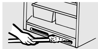
Clean the condenser coils at least once a year.
