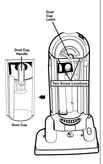
1. Remove dust cup from unit to expose the two screw installation locations. Release the dust cup by rotating the dust cup latch to the left. Pull out and up on the dust cup handle to remove from unit.
