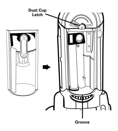
4. Replace dust cup by aligning front of the bottom of dust cup into groove on cleaner. Pivot dust cup up against cleaner and rotate the dust cup latch to the right to secure.
