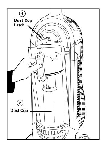
Release dust cup by rotating dust cup latch to the left pointing to the unlock symbol (3). Pivot dust cup out and away from cleaner and remove.
