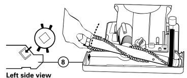
9. Align left end cap with square in base. Push end cap into place; see left side view.
