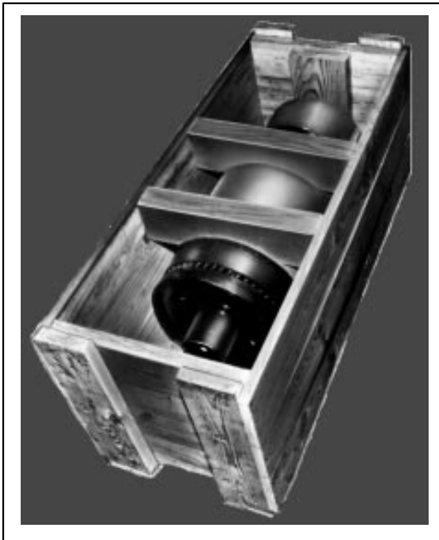
FIG. 47. SHIPPING BOX WITH ARMATURE, LESS COVER. E-3784.
